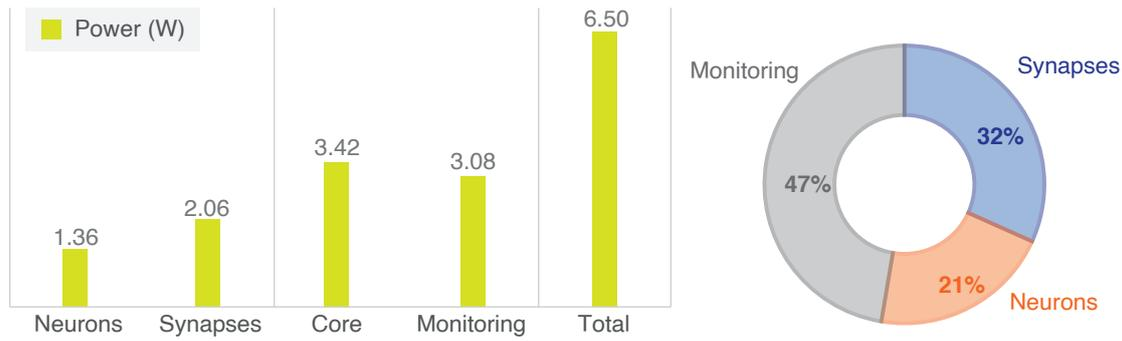
**Figure 3.17:** Distributed power consumption for implementation on AMD Xilinx KR260 Robotic Starter Kit exported from Vivado 2022.2.
