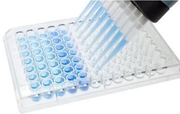
Figure 12: Assay manipulation in 96-well microtiter plate using a multichannel pipette.
