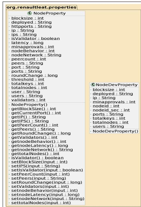
Figure 8.22: Simulation Property Module Package Architecture of Simulator
