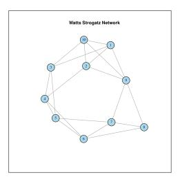
Figure 8.20: Watts Strogatz Network Topology of 10 Nodes
