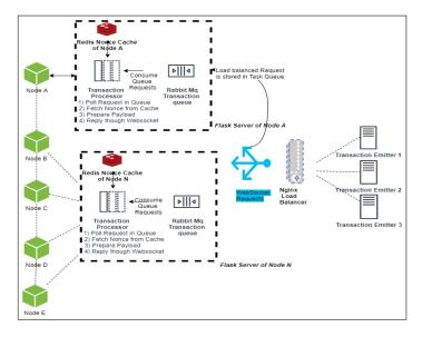
Figure 8.7: Ethereum Client Loadbalancer Middleware Architecture
