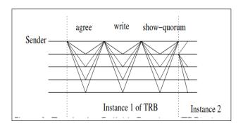
Figure 2.32: Terminating Reliable Broadcast Phases [138]
