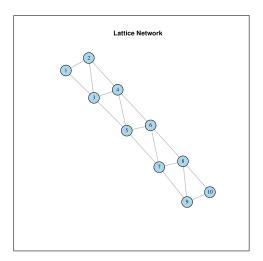
Figure 8.19: Lattice Network Topology of 10 Nodes
