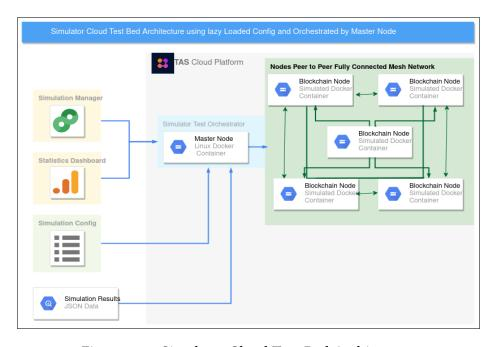
Figure 4.14: Simulator Cloud Test-Bed Architecture
