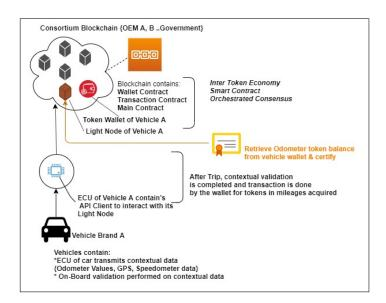
Figure 3.2: Non-Fungible Token Data Certification Architecture
