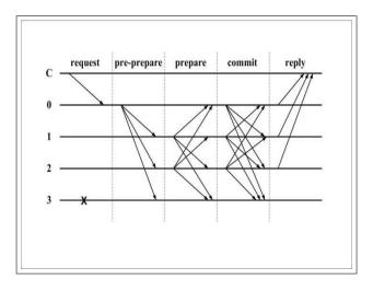
Figure 2.10: PBFT: Normal Case Operation [73]
