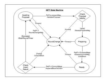
Figure 2.25: Istanbul Byzantine Fault Tolerance (IBFT) Consensus [119]
