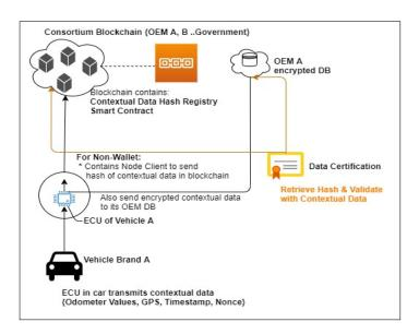
Figure 3.1: Data-Registry Data Certification Architecture
