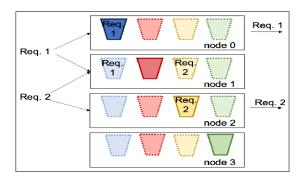
Figure 2.17: Sorting of Request into Buckets [94]
