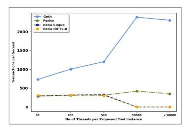
Figure 8.2: Custom Client Test Tool Thread Variation Performance
