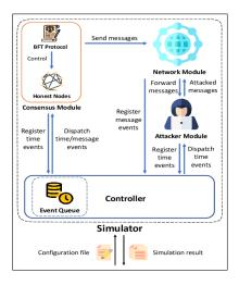
Figure 4.7: BFT Simulator Tool Infrastructure [190]
