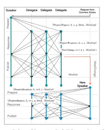
Figure 2.20: Delegated Byzantine Fault Tolerance Protocol [101]
