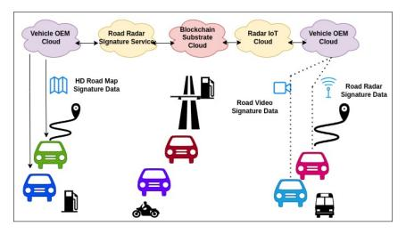
Figure 3.15: Automotive Road RADAR Signature Use Case
