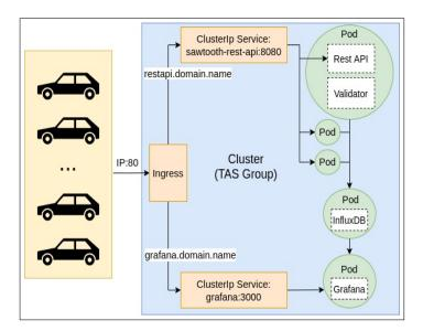
Figure 3.5: Hyperledger Sawtooth network cloud deployment
