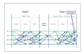
Figure 2.26: Quorum Byzantine Fault Tolerance (QBFT) Consensus [120],[121]
