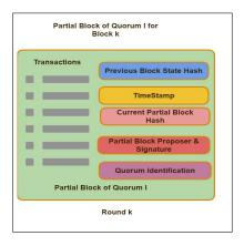
Figure 5.10: Partial Block Data Structure
