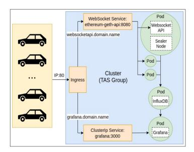
Figure 3.4: Ethereum network cloud deployment
