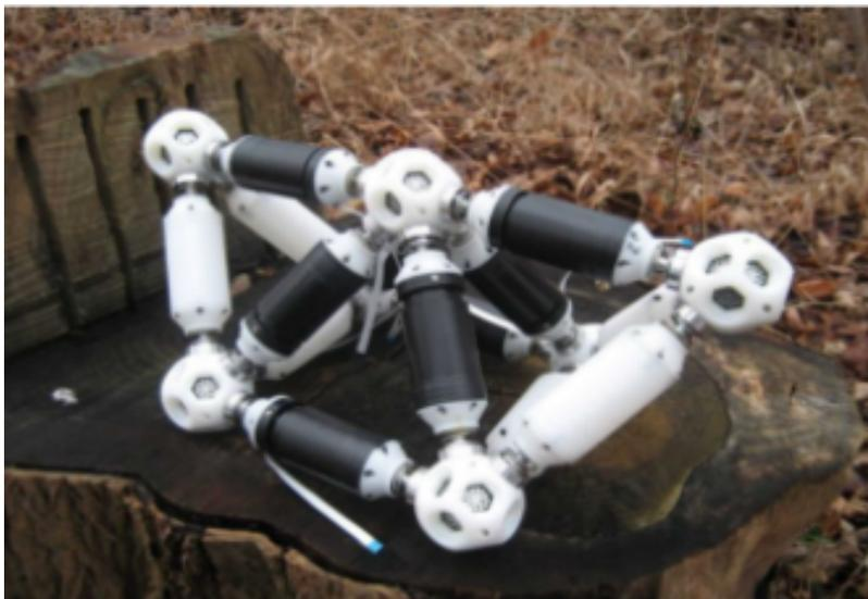
FIGURE 2.9: A truss structured system, Odin.
