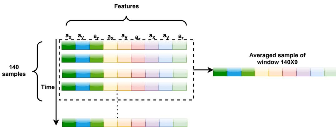
FIGURE 4.3: Averaged-window format for the proposed transformer model.
