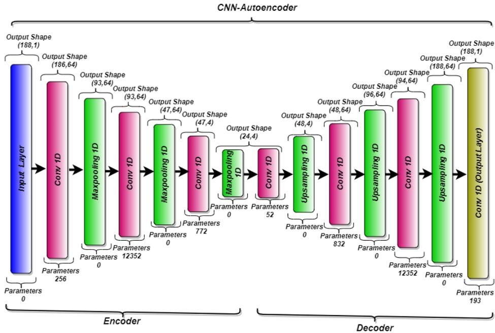
FIGURE 3.2: The architecture of the proposed denoising autoencoder
