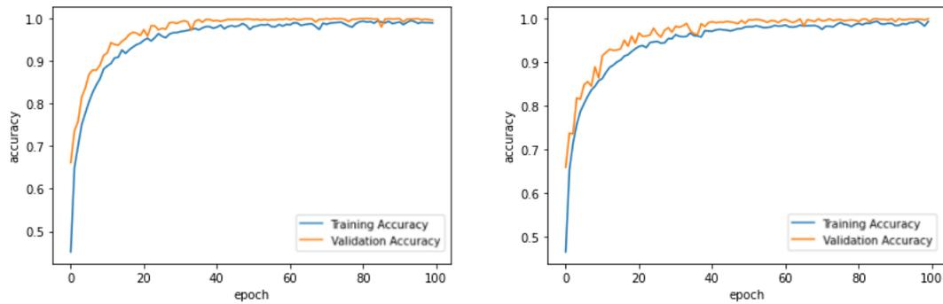
(A) Accuracy of the centralized model with the WISDM dataset
