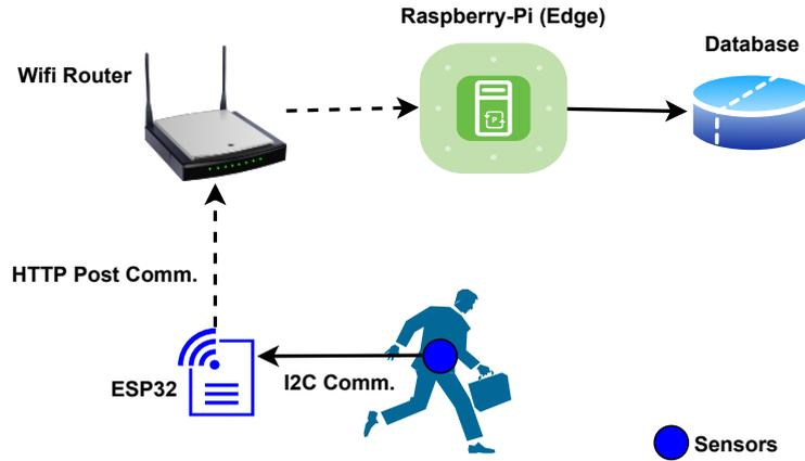
FIGURE 4.5: Our prototype for real-time data collection.
