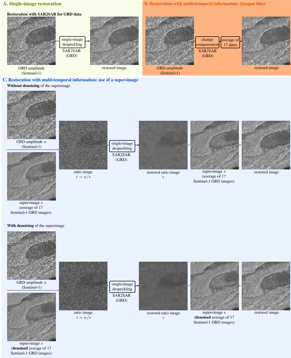
Figure 5.3: Comparison of several despeckling strategies for single-image and multi-temporal processing of GRD images. (A) Single image restoration: the SAR2SAR network is trained on GRD images and no temporal information is used. The estimated reflectivities are blurred and there is a lack of details. (B) Restoration with multi-temporal information and Quegan filter: despeckling based on temporal averaging with change compensated images. The SAR2SAR network is used to compute pre-estimated reflectivities to perform the change compensation. (C) Restoration with multi-temporal information and the use of super-image: the RABASAR based method. Two computations of the super-image are illustrated, the first one with simple temporal averaging and the second one with an additional denoising step of the temporal mean. The ratio image is computed and despeckled with SAR2SAR. With both computations of the super-image, the estimated reflectivities are sharper and contain more details. The higher the number of images in a stack, the fewer differences are between the two estimations. Figure extracted from [76].
