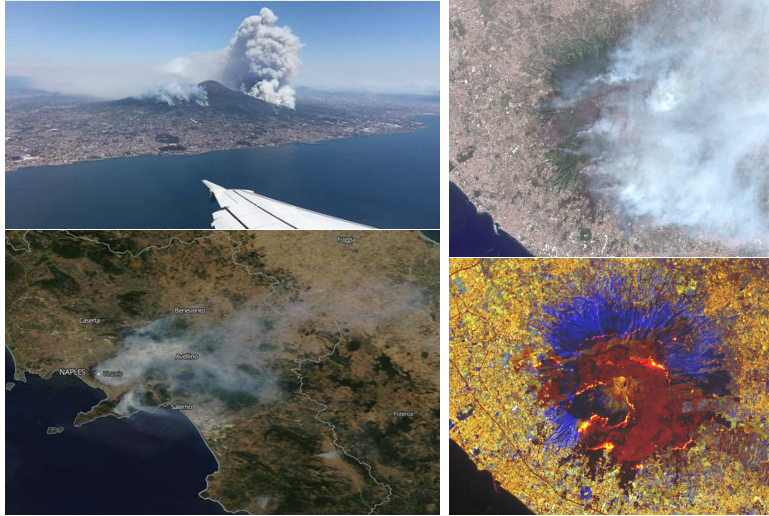
Figure 1.6: On the left panel, top: aerial view of the wildfires around the Vesuvio, bottom: MODIS (©NASA) image of the area. On the right panel, top: Sentinel-2 RGB image where only the smoke is visible, bottom: Sentinel-2 false color image obtained with Short-Wave Infrared and Near-Infrared bands where we can localize the points of high temperature i.e. the fire pits. Figure extracted from [4].
