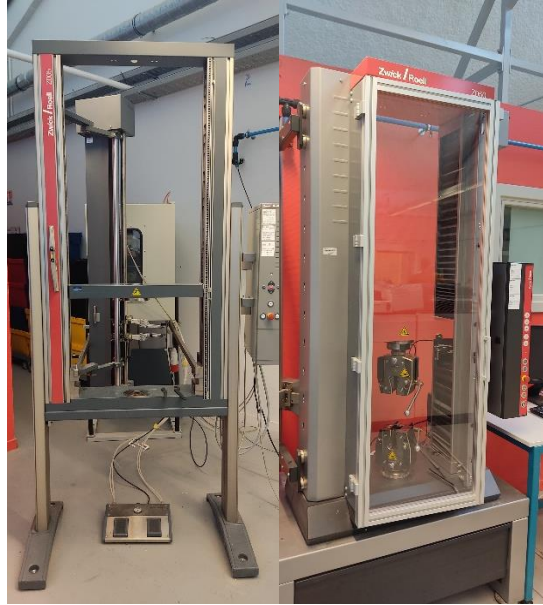
Figure 80: Mechanical testing machines (tensile, compression, flexure) at INSA Strasbourg, on the left-hand side, Zwick Roell® Z005 (maximum 5 kN), on the right-hand side, Zwick Roell® Z050 (maximum 50 kN)
