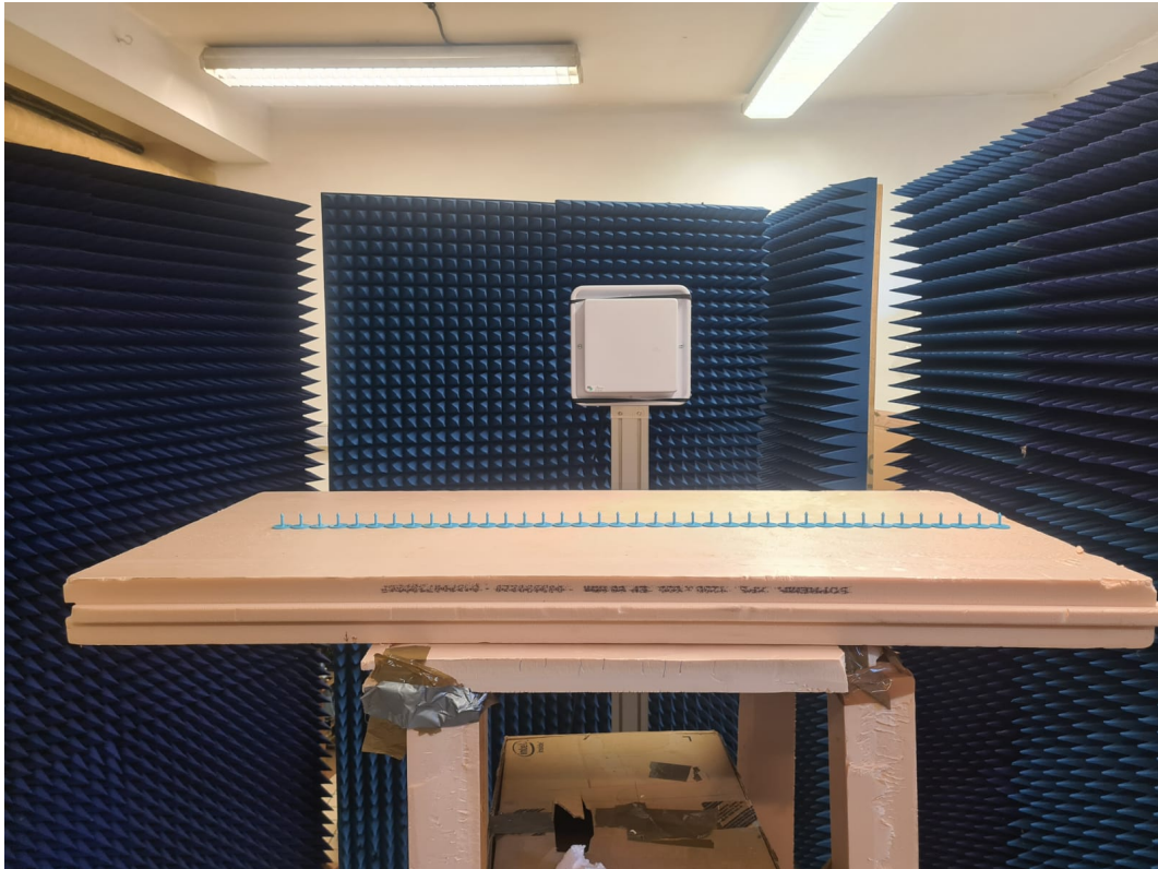
Figure 3.26 – Photo of the 39 tags placed in a row in front of the platform antenna surrounded by absorbent panels
