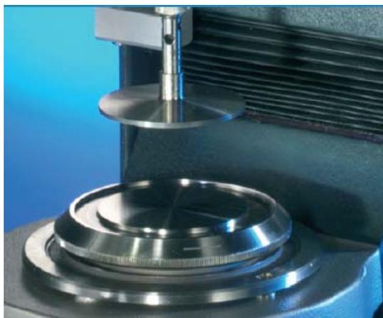
*Figure 1. The Haake Rheostress rheometer*
