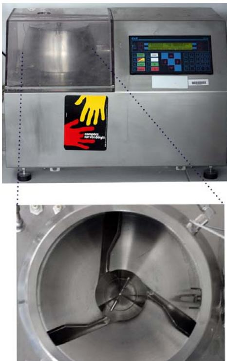
*Figure 23. The Diosna high shear mixer*
