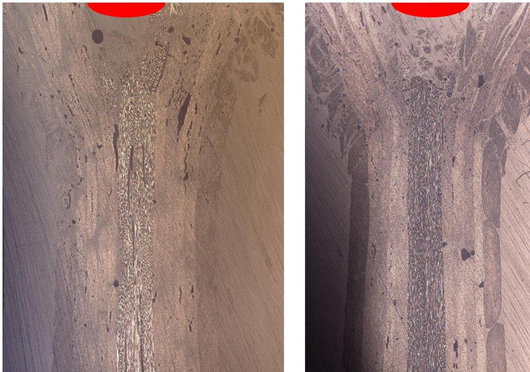
Figure 5.24 – Polished sections of unaged (left) and seawater saturated (right) coupons impacted at 330J
