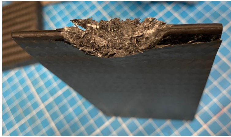
Figure 5.32 – Delamination of the external ply due to the impact at 100J
