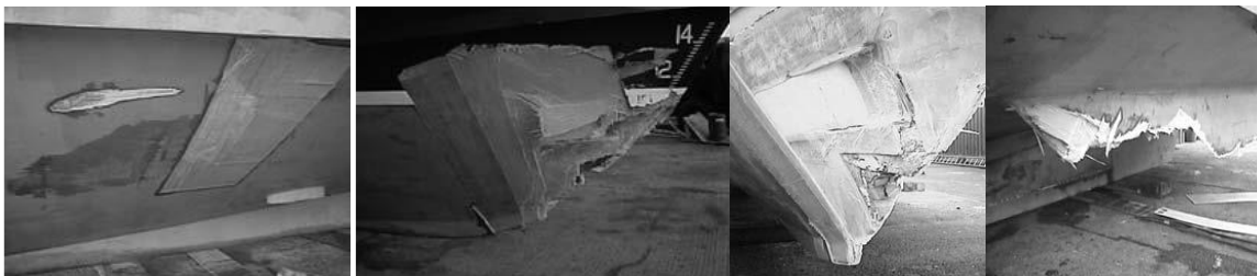
Figure 1.8 – Examples of structural damage on vessels due to marine impacts [91]
