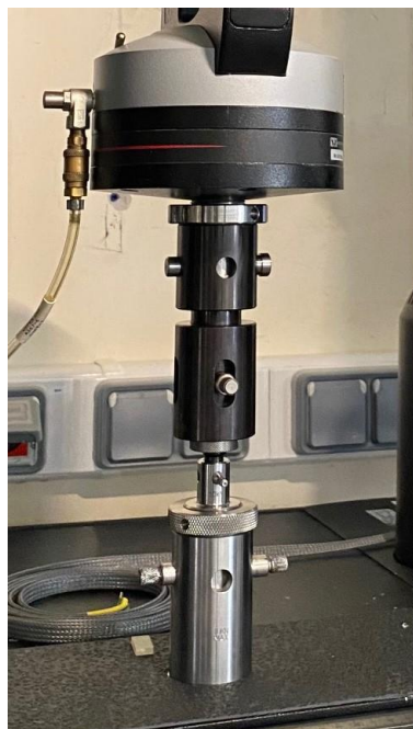
Figure 2.19 – Fixture used to load a coupon at the same loading–rate
