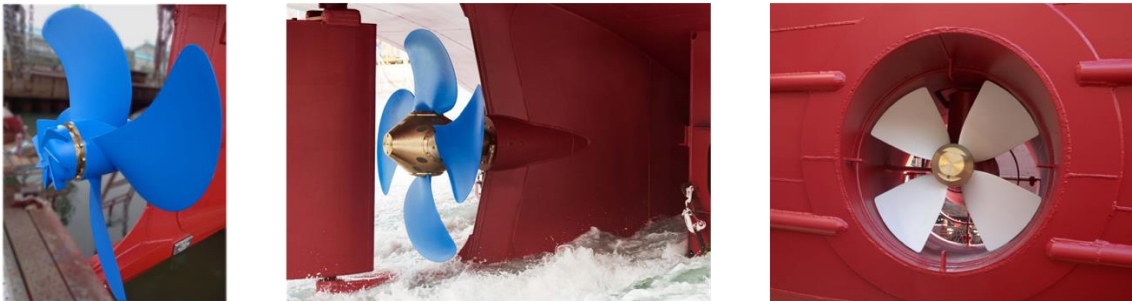
Figure 1.1 – CFRP marine propellers commercialized by Nakashima (from Nakashima website) – In the order : i) Fixed Pitch Propeller (FPP) ii) Controllable Pitch Propeller (CPP) iii) Side thruster
