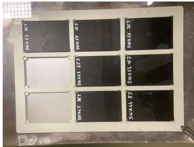
Figure 2.5 – Fixture designed for scanning several coupons at the same time
