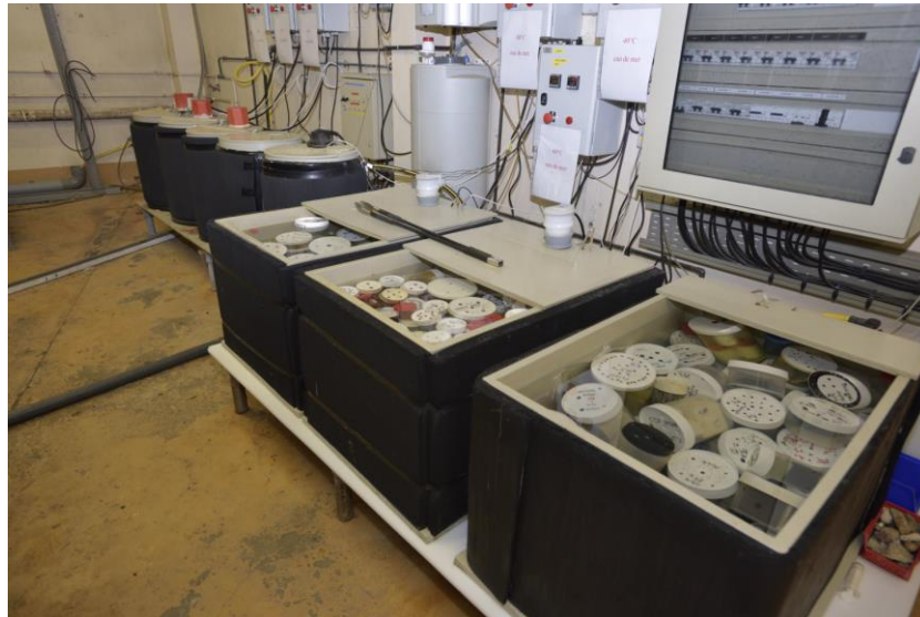
Figure 2.2 – Seawater aging tanks at IFREMER
