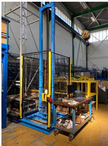
Figure 2.20 – IFREMER drop weight impact tower
