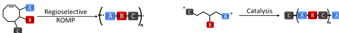
Figure 3: Examples of how a tailored synthesis of a monomer and the choice of the polymerization pathway can induce a sequence in the resulting polymer. On the left: cyclooctene bearing different functional groups undergoes ring-opening metathesis polymerization (ROMP) to produce a periodic copolymer. On the right: designed monomers bearing polymerizable functional groups (*) can give similar periodic copolymers.
