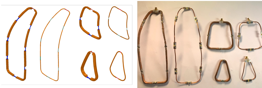
Figure 3.10: Simulation model of the loops with "U" and cylindrical sections (left), modeled with lossy capacitors; 3D printed loops and the handmade copper wire equivalents (right).
