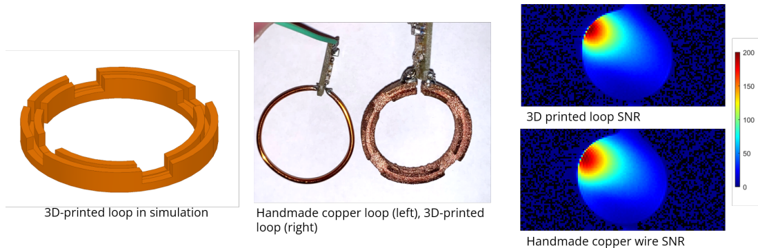
Figure 3.6: A small 3D-printed loop of 3-cm diameter is compared to a regular handmade copper wire. The SNR from the loops as measured in the scanner is equivalent between the two loops (in the same conditions and with the same preamplifier).
