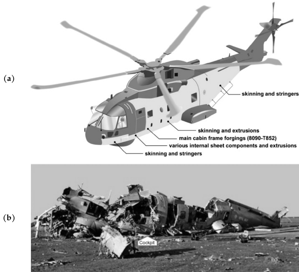
FIGURE I.17: Agusta–Westland EH101 helicopter early model: (a) components made of Al–Li alloys (Pasang et al., 2012); (b) hard landing due to a tail-rotor failure attributed the low toughness of alloy 8090 (Wanhill et al., 2013).
