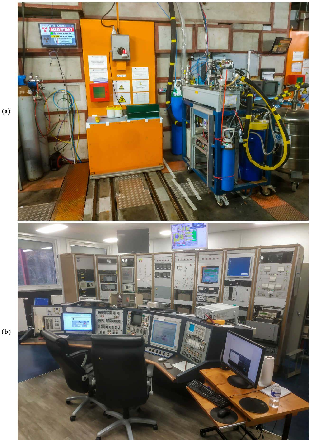
FIGURE III.56: Cyclotron of CEMHTI: (a) exterior view of the irradiation cell whose entry is closed by a reinforced door, with the helium gas cooling and purification system on the right-hand side; (b) control room of the cyclotron, which continuously require two operators.
