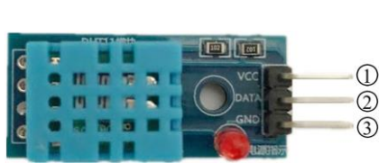
Figure 4.19 DHT11 temperature and humidity module
