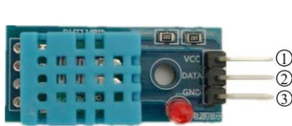
Figure 4.19 DHT11 temperature and humidity module
