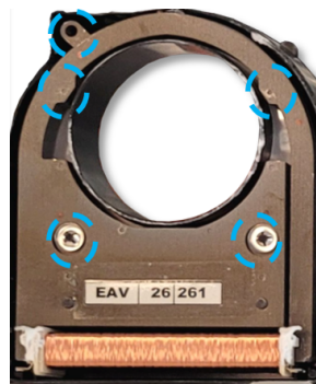
Figure IV.10: Masterpact MTZ current transformer, geometry elements in blue that are simplified in the simulation model.
