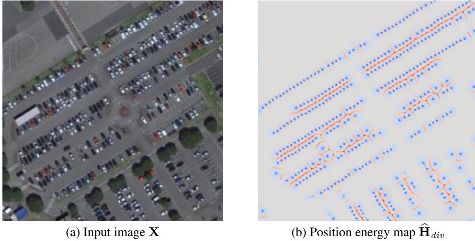
Figure 4.9: Example of inferred energy map. Image from DOTA (Xia et al., 2018) with corresponding inferred energy map. Blue areas corresponds to negative potentials while red to positive potentials.
