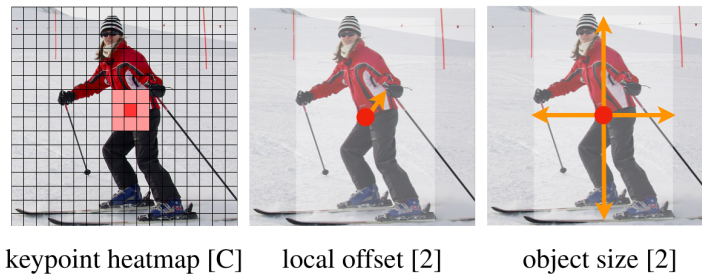
Figure 2.4: Heatmap for center detection. Here the heatmap resolution is coarser than the image resolution, the local offset allows compensating for the discretization error. From (X. Zhou et al., 2019).
