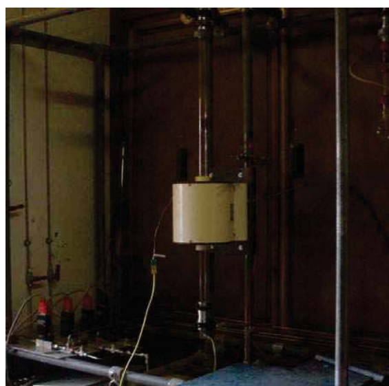
Figure 1: Vertical reactor for carbonaceous nanomaterials synthesis
