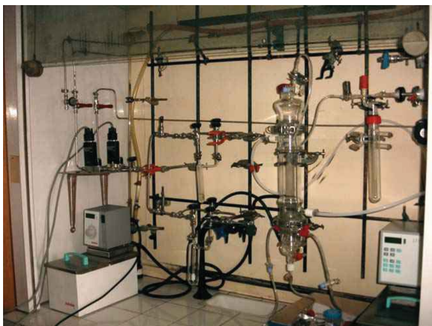
Figure 3: FB-CVD apparatus for the catalysts elaboration
