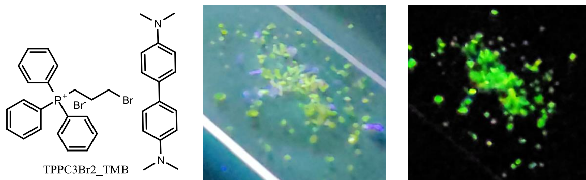
Figure 5.8. Shows a crystal of TPPC3Br 2 _TMB, with the central image showing the crystal while under excitation and the image on the right showing the crystal right after the excitation source (wavelength 260 nm) has been turned off
