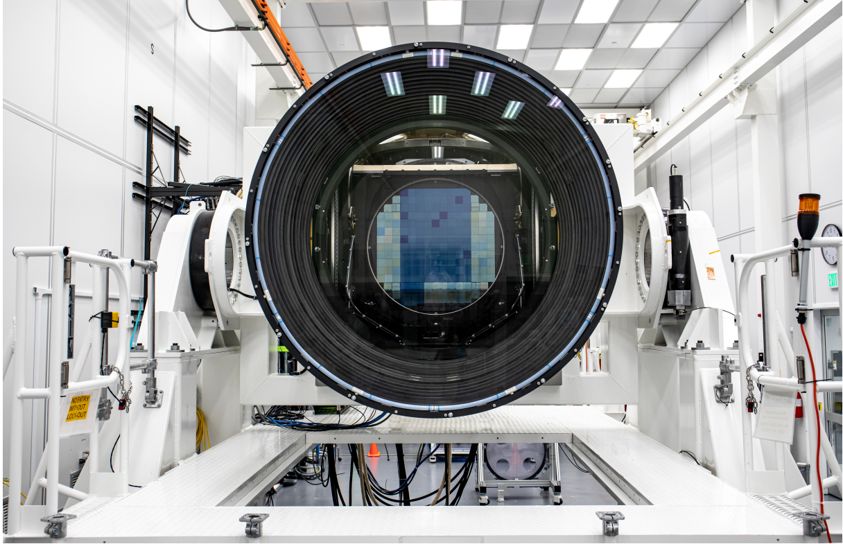
Figure 3.4: Front picture of the integrated LSST Camera located in the clean room at SLAC (front lens \sim 1.6 m). Credits https://www.lsst.org/ .
