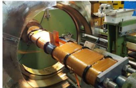
FIG. 2. Application of the mechanical reinforcement on the foil coil. Two 3D printed halves of a hollow cylinder, in black on the photo, containing four M24 stainless steel tie rods and filled with epoxy resin permit to wind the Zylon fibers and to transmit the force in the direction parallel to the fibers. Zylon fibers are wound over a length of 600 mm with a thickness of about 5 mm and are capable to sustain a force above 3000 tons, giving us a safety margin of about a factor 4, but also limiting the possible displacement of the layers to around a few tens of micrometers, decreasing the risk of buckling of the foils. At each end of the magnet, the mechanical stress is naturally transmitted as a hoop stress in the copper foil as the winding can be considered as two halves of a solenoid. The extremities of the magnet are reinforced with two 25 mm thick stainless steel plates that are also used to fix the magnet, screwed with the M24 tie rods.
