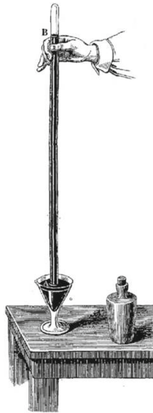
Fig. 3 Torricelli's experiment. A tube filled with mercury is turned upside down inside a container filled of the same liquid. One observes that the level of the mercury in the tube decreases and stops at a fixed height. The space at the top of the glass tube is no more filled with mercury. Is it a vacuum? Illustration extracted from Ganot [39]
