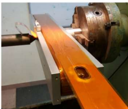
FIG. 1. Photo of the foil coil during the winding showing one hole in the copper foil and in the Kapton tape. The holes have a racetrack shape to keep a circular access when the foil is wound over the round end of the magnet. The copper is cut first, and then, the insulation with the Kapton tape is cut with a smaller hole to ensure a perfect electrical insulation between two layers thanks to the overlapping of the Kapton on the copper.
