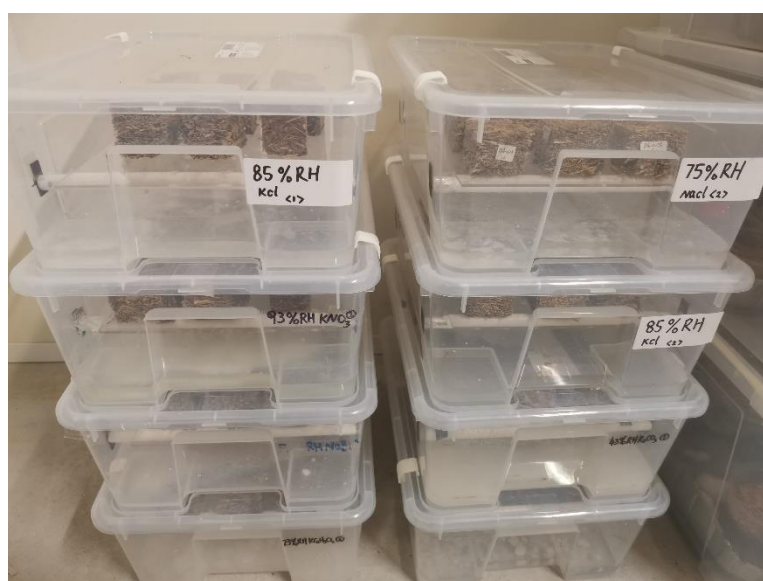
Figure 3.15. Experimental setup for the saturated salt solution method
