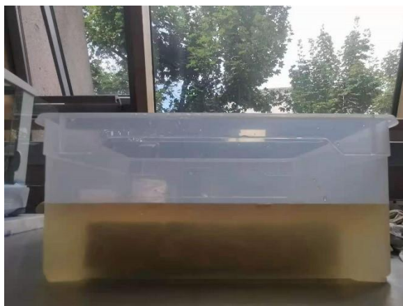
Figure 3.8. Immersion alginate-based composite in \text{CaCl}_2 solution
