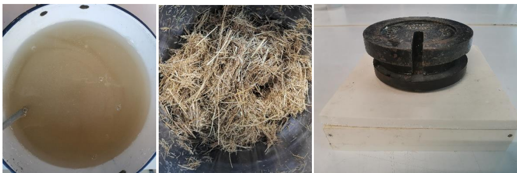
Figure 3.7. Binder solution (left), wet fibres (middle) and compression by weight (right)
