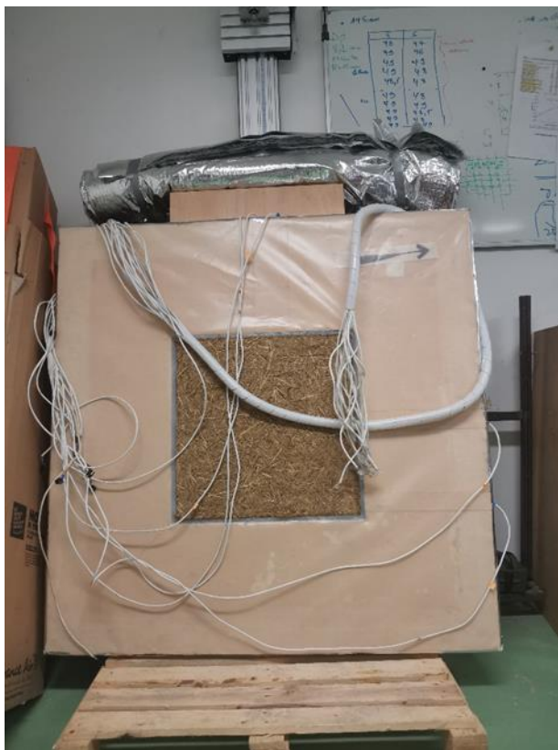
Figure 4.5. Whole assembly of the tested wall
