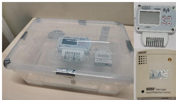
Figure 3.14. HOBO sensors for measuring the relative humidity in the salt box
