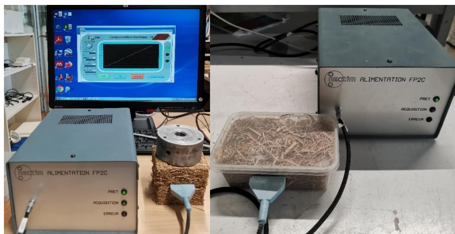
Figure 3.11. Thermal conductivity and effusivity measurements for fibers and composites
