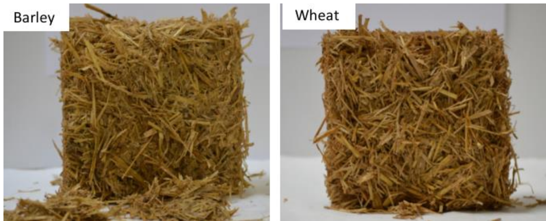
Figure 2.7. State of barley and wheat straw composites after 35 and 40 drying-wetting cycles respectively
