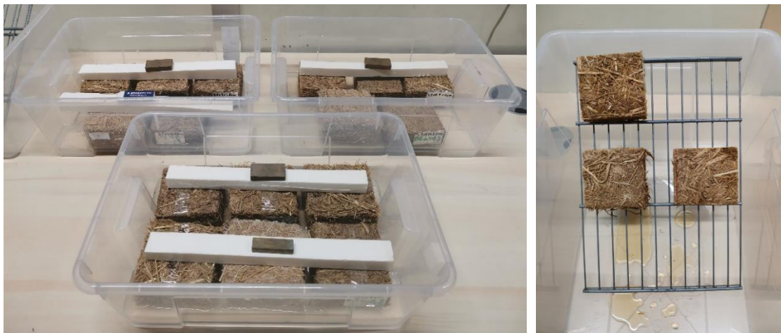
Figure 3.16. Water absorption test
