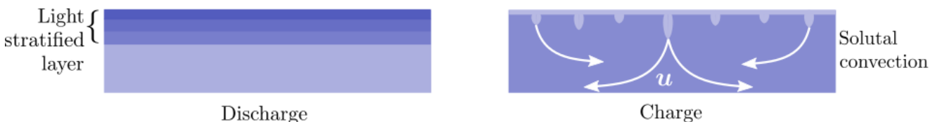
Figure 1.8 – Effect of solutal buoyancy in LMBs: scheme of the concentration distribution of light metal A in the alloy during discharge and charge.
