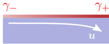
Figure 6.1 – Scheme representing a Marangoni flow due to spatial gradients of surface tension at a surface.
