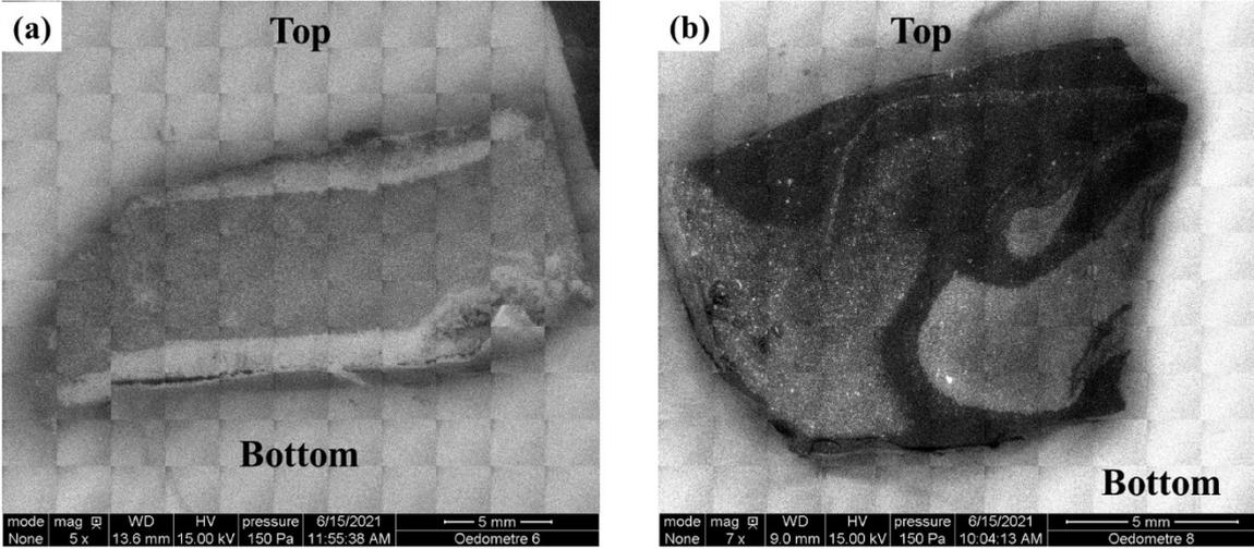
Fig. 3-16 ESEM observation of the cross-sections of BWPs containing 30 wt. % NaNO<sub>3</sub> under constant counter-pressure of (a): 176kPa (5 x magnification) after 683 days of leaching; (b) 2.8 MPa (7 x magnification) after 683 days of leaching.
