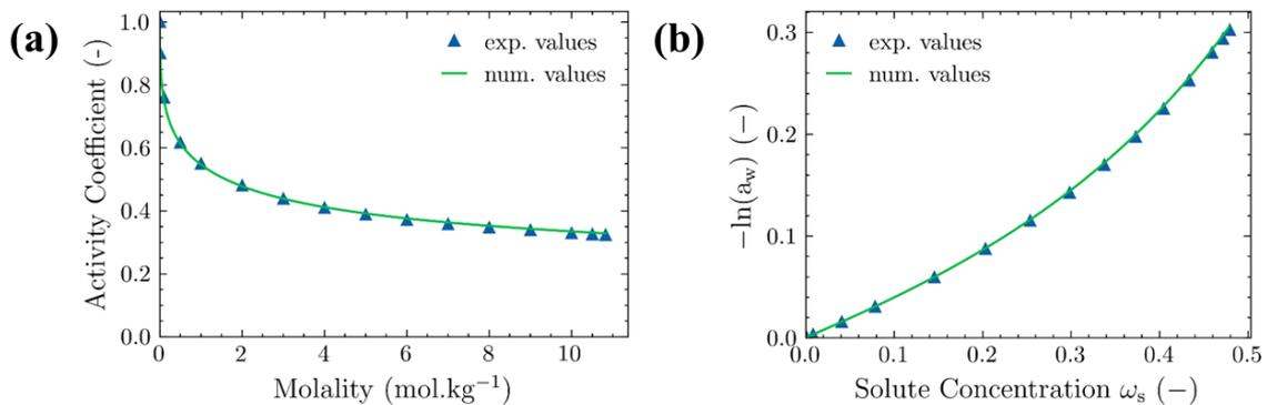
Fig. 5-31 Numerical values of (a) salt activity coefficient; (b)  $-\ln(a_w)$  simulated with the fitted Pitzer's model parameters listed in Table 10. The experimental values are respectively from [47] and [35].
