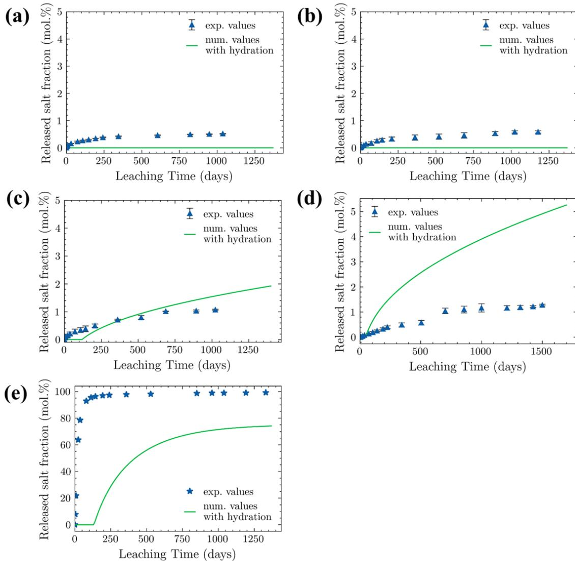
Fig. 5-19 Numerical and experimental results of the amount of leached salts for (a) M5\_NaNO3; (b) M10\_NaNO3 ; (c) M20\_NaNO3; (d) M30\_NaNO3 BWPs; (e) M5\_NaNO3\_M35\_BaSO4.
