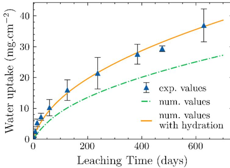
Fig. 5-12 Numerical and experimental results of the temporal evolution of absorbed water of M10\_Na<sub>2</sub>SO<sub>4</sub> mono-salt BWP.
