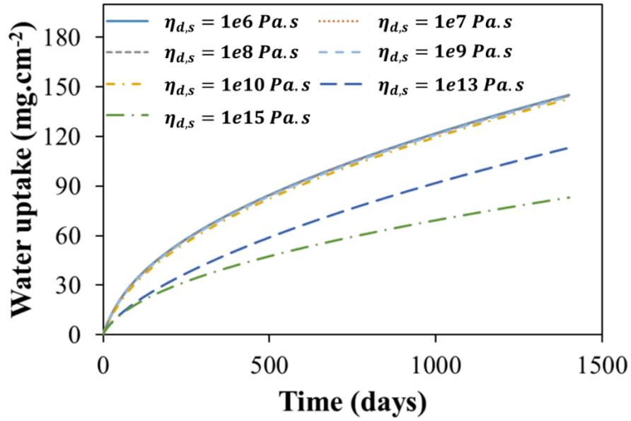
Fig. E - 6 Temporal evolutions of water uptake amounts for M20\_NaNO3 BWPs under free leaching conditions with deviatoric viscosity  $\eta_{d,s}$  ranging from  $\eta_{d,s} = 1 \times 10^6 \text{ Pa.s}$  to  $\eta_{d,s} = 1 \times 10^{15} \text{ Pa.s}$ .
