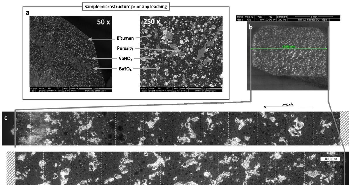
Fig. 3-11 ESEM observation of a BWP sample containing 5 wt. % NaNO<sub>3</sub> and 35 wt. % BaSO<sub>4</sub>: (a) Sound before any leaching experiment (50 x and 250 x magnifications); (b) Overview of the cross-section of a sample after 1000 days of leaching (14 x
