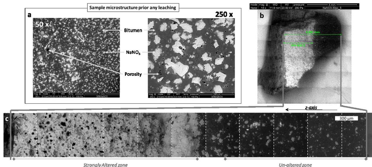
Fig. 3-9 ESEM observation of a BWP containing 30 wt. % NaNO<sub>3</sub>: (a) Sound before any leaching experiment (50 X and 250 X magnification); (b) Overview of the cross-section of a sample after 1400 days of leaching (14 x magnification); (c) Z profile reconstruction along the leached sample cross section after 1400 days of leaching (200 x magnification).
