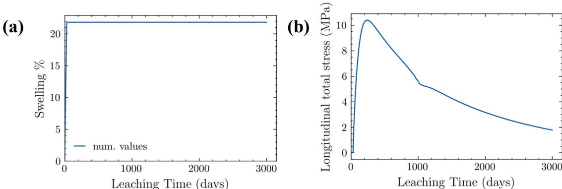
Fig. 5-41 (a) Temporal evolution of swelling ; (b) stress build-up behavior for the case of free leaching followed by leaching under constant volume conditions simulated on a 2.5 mm high bi-salt M10\_NaNO3\_M30\_BaSO4. A swelling of 22 vol. % is allowed under free leaching conditions. The bi-salt parameters fitted on M10\_NaNO3\_M30\_BaSO4 under free leaching conditions (cf. Table 19) are used.
