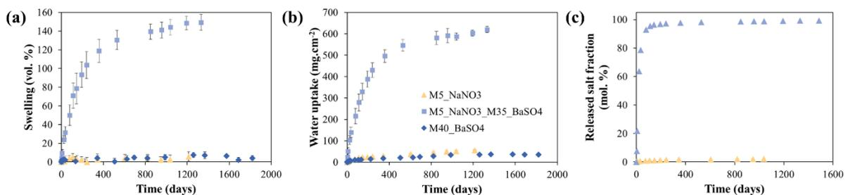
Fig. 3-8 Comparison of (a) swelling (vol. %); (b) water uptake ( $\text{mg}/\text{cm}^2$ ); (c) released salt fraction (mol. %) between mono-salt M5\_NaNO<sub>3</sub> BWP, M40\_BaSO<sub>4</sub> BWP and bi-salt M5\_NaNO<sub>3</sub>\_M35\_BaSO<sub>4</sub> BWP.
