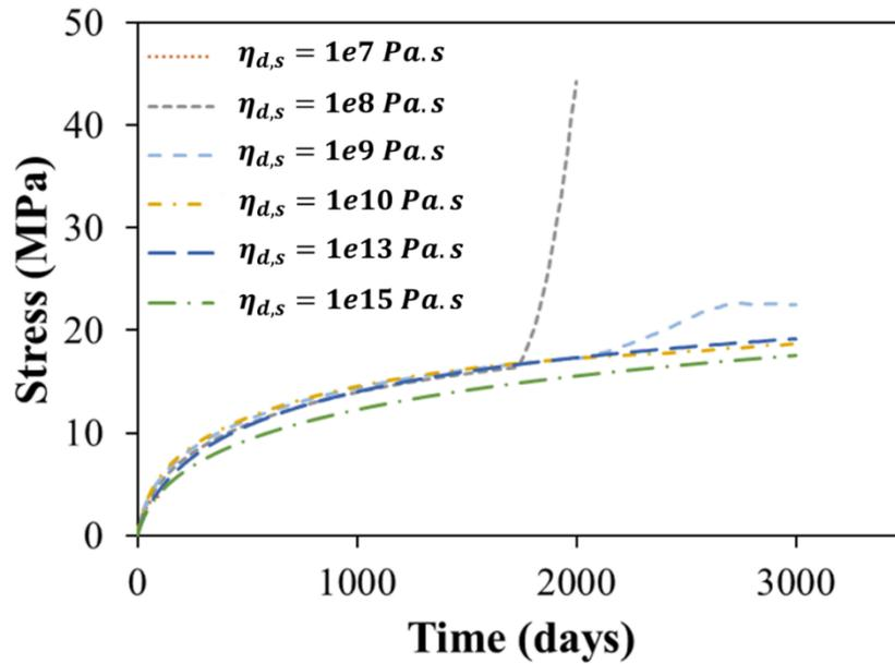
Fig. E - 3 Temporal evolutions of generated stress simulated for M20\_NaNO3 BWPs under constant volume conditions with deviatoric viscosity  $\eta_{d,s}$  ranging from  $\eta_{d,s} = 1 \times 10^7 \text{ Pa}\cdot\text{s}$  to  $\eta_{d,s} = 1 \times 10^{15} \text{ Pa}\cdot\text{s}$ .
