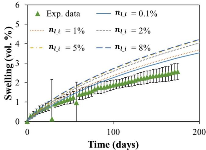
Fig. 5-28 Swelling behavior under 176 kPa constant counter-pressure of M10\_NaNO<sub>3</sub>\_M30\_BaSO<sub>4</sub> BWP with different initial porosity  $n_{L_i}$ . The numerical results are compared with the average of the experimental results shown in Fig. 3-17.
