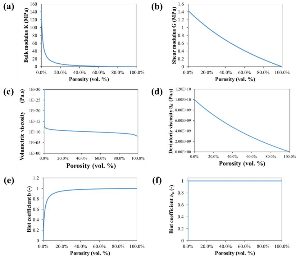
Fig. 4-3 Evolution in terms of porosity of (a) bulk modulus  $K$ ; (b) shear modulus  $G$ ; (c) volumetric viscosity  $\eta_v$  (plotted in logarithmic scale of 10); (d) deviatoric viscosity  $\eta_d$ ; (e) Biot coefficient  $b$ ; (f) viscous Biot coefficient  $b^v$ .
