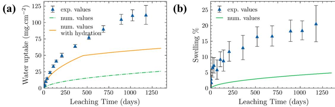
Fig. 5-4 Numerical and experimental results of the temporal evolution of (a) absorbed water; (b) swelling of M20\_  $\text{NaNO}_3$  mono-salt BWP using the MELOT2019 model and parameters reported in [1,2].
