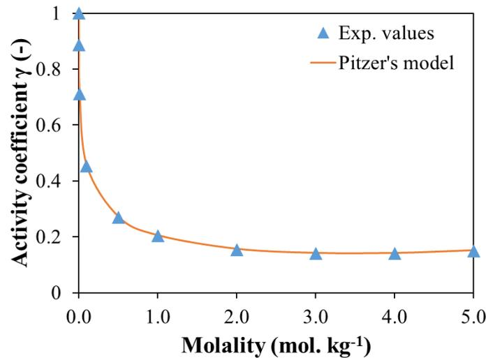
Fig. A - 2 Comparison of experimental data [56] and activity coefficients calculated with Pitzer's model and parameters reported for the aqueous solution of  $\text{Na}_2\text{SO}_4$  at 25°C (cf. Table A. 1).
