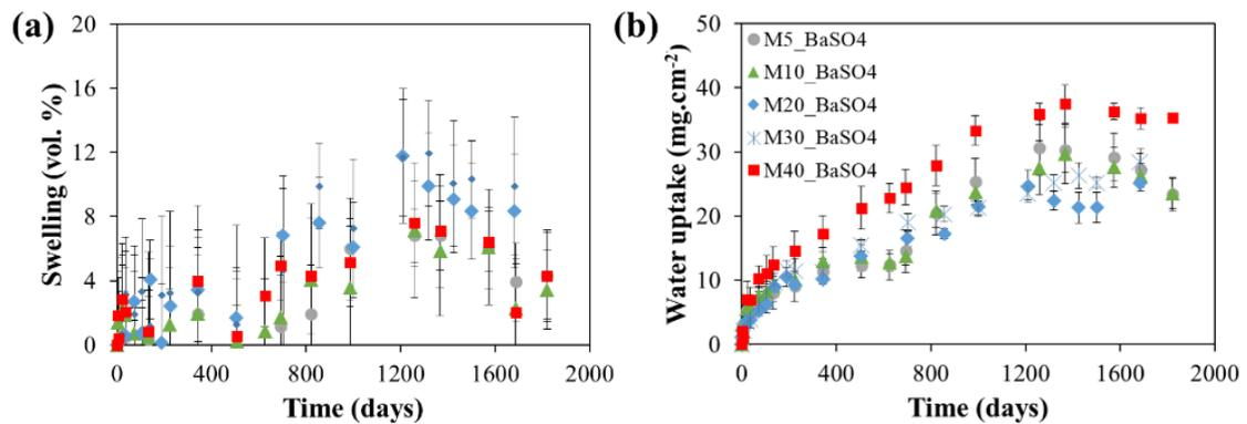
Fig. 3-6 Experimental measurements of (a) swelling (vol. %); (b) water uptake ( $\text{mg}/\text{cm}^2$ ) during free leaching tests of mono-salt BWPs containing 5 wt.%, 10 wt.%, 20 wt.%, 30 wt.% and 40 wt.% of  $\text{BaSO}_4$ .
