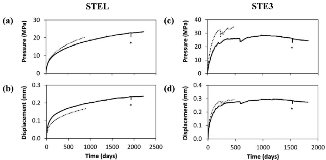
Fig. 2-9 Evolution of the generated pressure and displacement as a function of time after leaching of STEL (a-b) and STE3 (c-d) samples under nearly constant volume conditions. \*: pressure and displacement decreases caused by a temperature decrease in the lab during a power failure [17].
