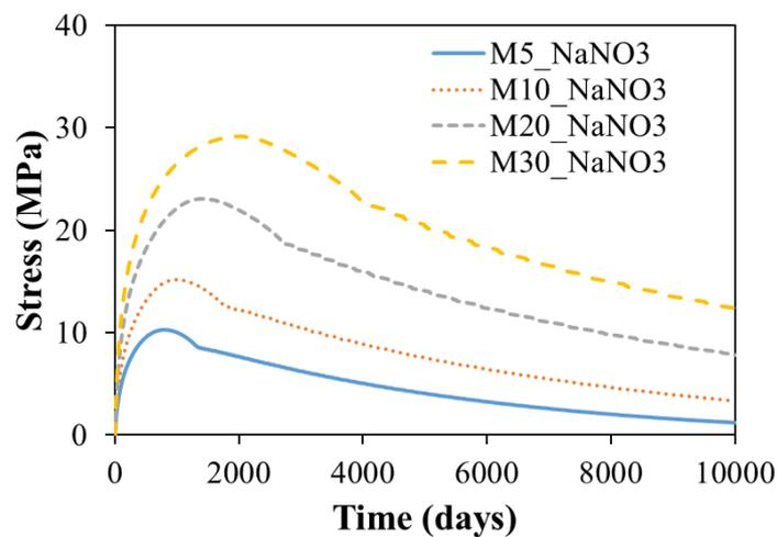
Fig. 5-34 Evolution of stress generated over leaching time within mono-salt NaNO<sub>3</sub> BWPs containing 5, 10, 20 and 30 wt. % of NaNO<sub>3</sub>.
