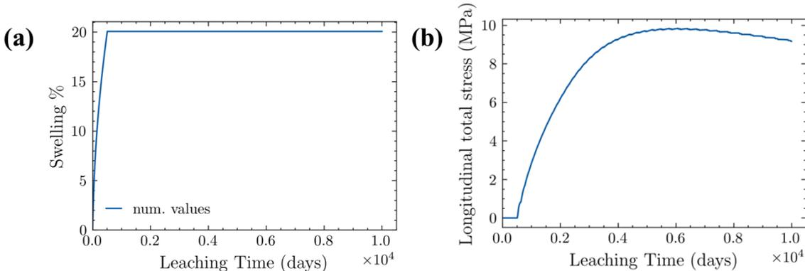
Fig. 5-40 (a) Temporal evolution of swelling ; (b) stress build-up behavior for the case of free leaching followed by leaching under constant volume conditions simulated on a 2.5 mm high bi-salt M10\_NaNO3\_M30\_BaSO4. A swelling of 20 vol. % is allowed under free leaching conditions. The mono-salt parameters (cf. Table 18) are used.
