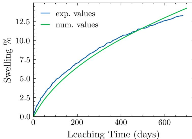
Fig. 5-23 Numerical and experimental results of the temporal evolution of swelling of M30\_NaNO<sub>3</sub> mono-salt BWP under 176 kPa constant counter-pressure.
