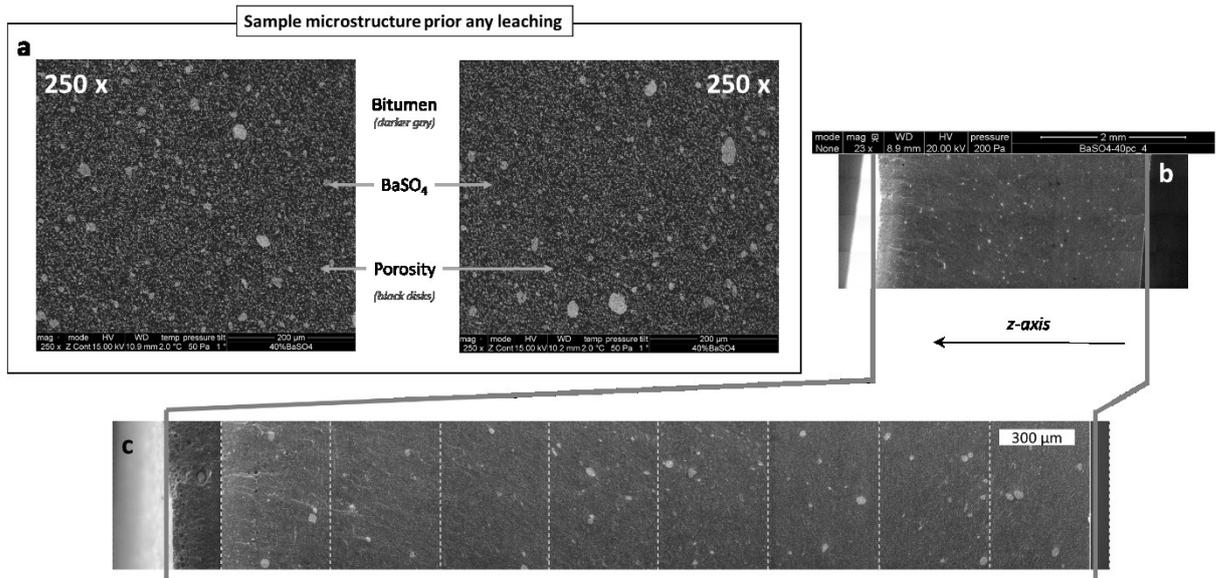
Fig. 3-10 ESEM observation of a BWP sample containing 40 wt. % BaSO<sub>4</sub>: (a) Sound before any leaching experiment (250 X magnification at two different locations); (b) Overview of the cross-section of a sample after 1400 days of leaching (14 x magnification); (c) Z profile reconstruction along the leached sample cross section after 1400 days of leaching (200 x magnification)
