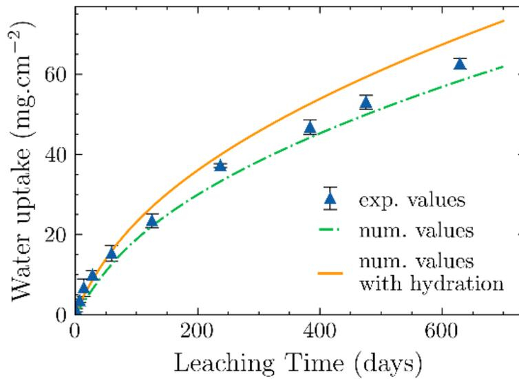
Fig. 5-13 Numerical and experimental results of the temporal evolution of absorbed water of M25\_Na<sub>2</sub>SO<sub>4</sub> mono-salt BWP.
