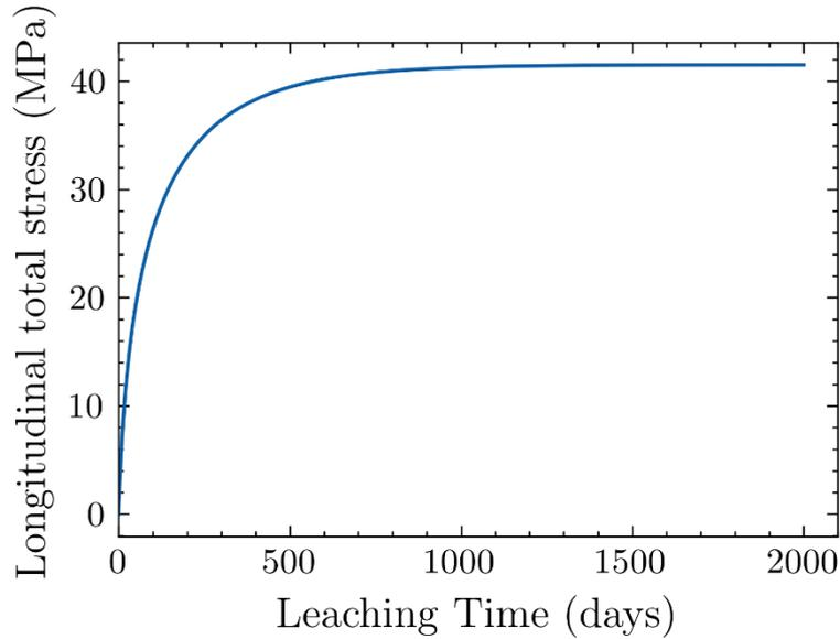
Fig. 5-29 Stress build-up behavior of mono-salt  $\text{NaNO}_3$  BWPs under constant volume conditions with a perfect semi-permeable membrane simulated with the fitted Pitzer's model parameters listed in Table 10.
