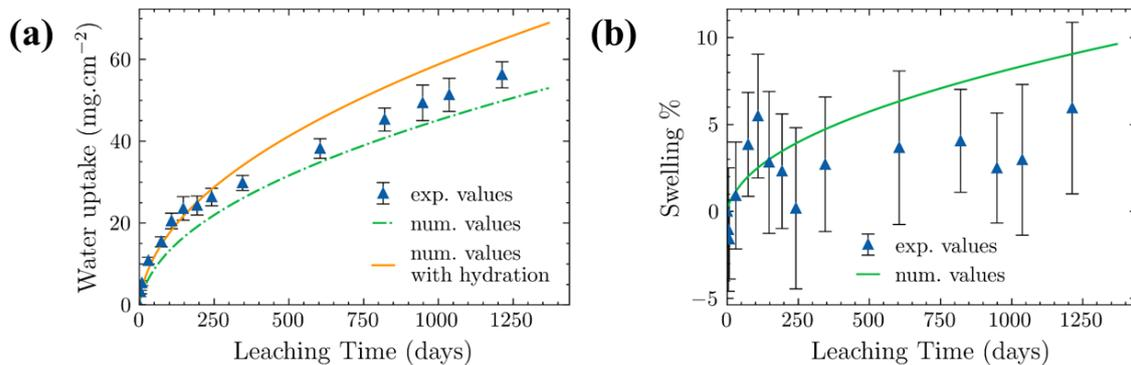
Fig. 5-8 Numerical and experimental results of the temporal evolution of (a) absorbed water; (b) swelling of M5\_NaNO<sub>3</sub> mono-salt BWP.
