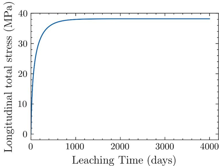
Fig. 5-32 Stress build-up behavior of mono-salt  $\text{NaNO}_3$  BWPs under constant volume conditions with a perfect semi-permeable membrane simulated with Pitzer's model parameters reported in [47] and listed in Table 22.
