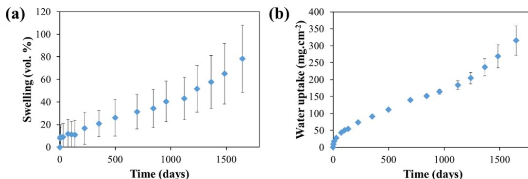
Fig. 3-12 Experimental measurements of (a) swelling (vol. %); (b) water uptake (mg/cm<sup>2</sup>) during free leaching tests on industrial BWP STE3.
