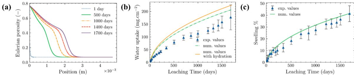
Fig. 5-10 (a) Profile along the sample of porosity at different leaching times. Numerical and experimental results of the temporal evolution of (b) absorbed water; (c) swelling of M30\_NaNO<sub>3</sub> mono-salt BWP.
