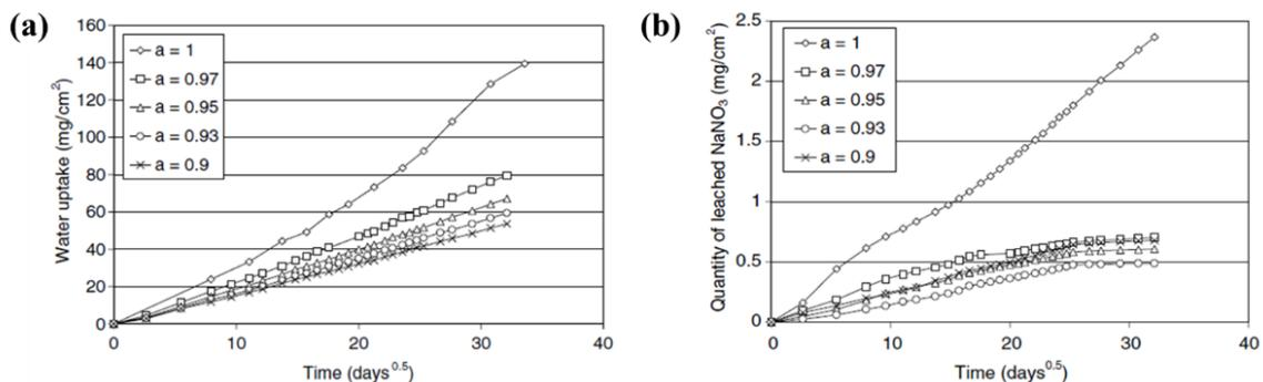
Fig. 2-4 Experimental measurements of (a) water uptake ( $\text{mg}/\text{cm}^2$ ); (b) released  $\text{NaNO}_3$  ( $\text{mg}/\text{cm}^2$ ) of STE3 leached by solutions with water activity  $a$  ranging from 0.9 to 1 [15].
