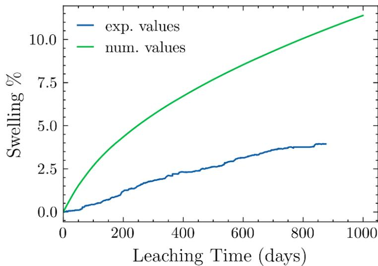
Fig. 5-26 Numerical and experimental results of the temporal evolution of swelling of M30\_NaNO<sub>3</sub> mono-salt BWP under 2.8 MPa constant counter-pressure.
