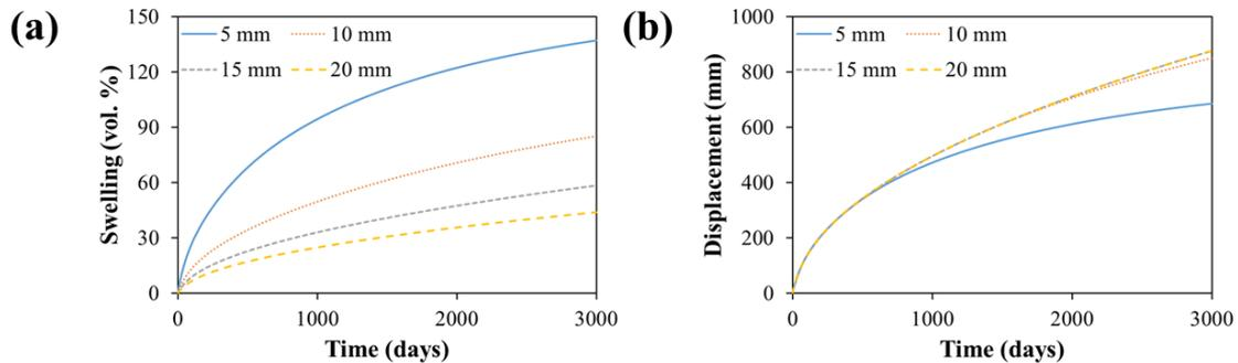
Fig. 5-20 Temporal evolution of (a) swelling ; (b) displacement of M10\_NaNO3\_M30\_BaSO4 BWPs simulated with sample height ranging from 5 mm to 20 mm.
