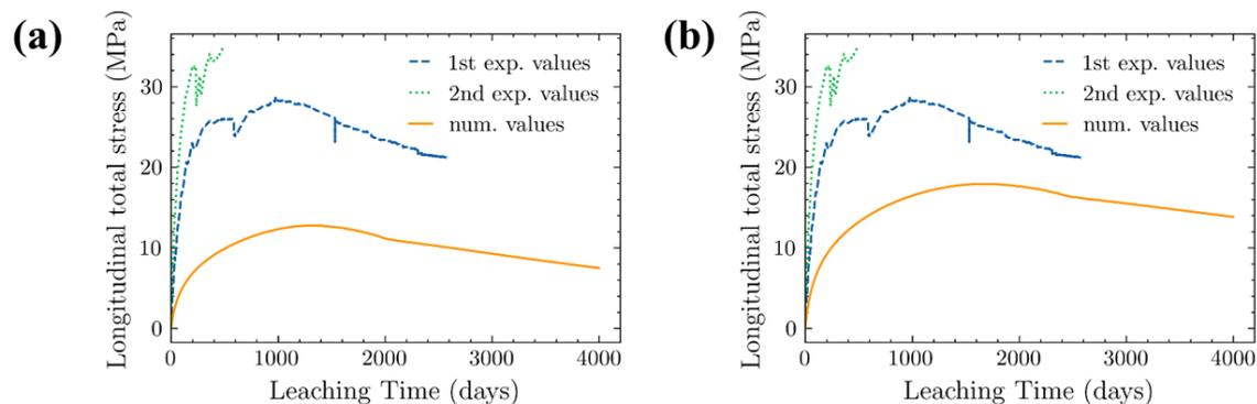
Fig. 5-47 Comparison of experimental results from [17] and numerical simulation of the stress build-up behavior of STE3 under constant volume conditions using (a) parameter set 1; (b) parameter set 2 in Table 25.
