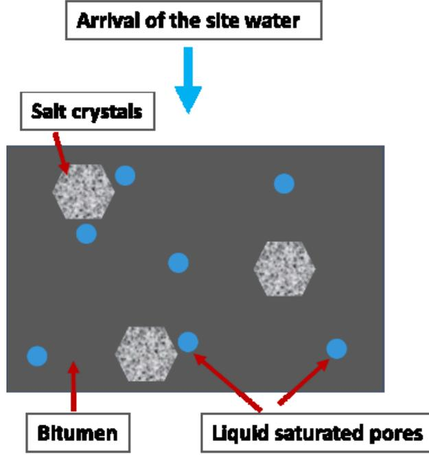
Fig. 4-1 Schematic representation of BWPs.
