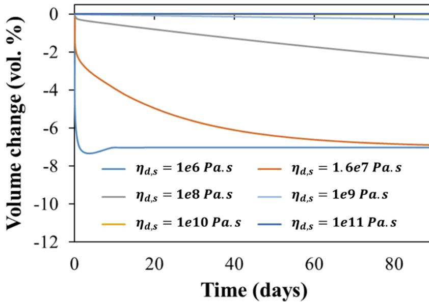
Fig. E - 2 Temporal evolutions of volume change simulated for M20\_NaNO3 BWPs consolidated under 100 Pa with deviatoric viscosity  $\eta_{d,s}$  ranging from  $\eta_{d,s} = 1 \times 10^6$  Pa.s to  $\eta_{d,s} = 1 \times 10^{11}$  Pa.s.
