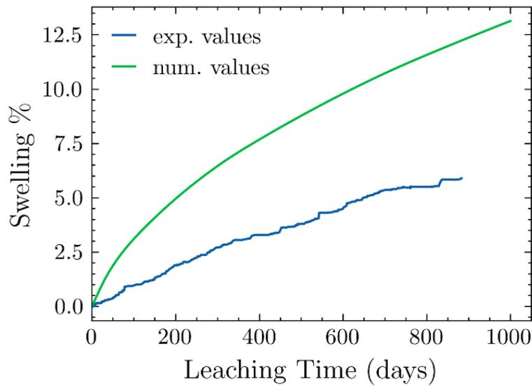
Fig. 5-25 Numerical and experimental results of the temporal evolution of swelling of M30\_NaNO<sub>3</sub> mono-salt BWP under 1.4 MPa constant counter-pressure.
