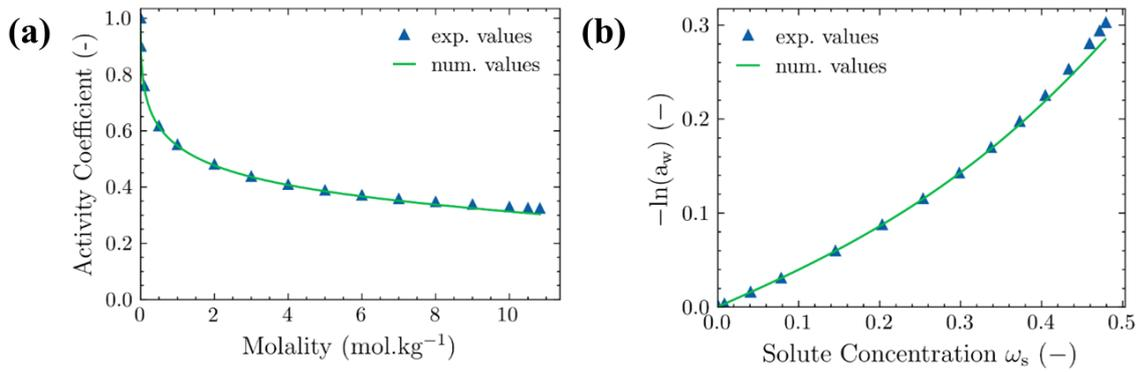
Fig. 5-33 Numerical values of (a) salt activity coefficient; (b)  $-\ln(a_w)$  simulated with the fitted Pitzer's model parameters reported in [47] and listed in Table 22. The experimental values are respectively from [47] and [35].
