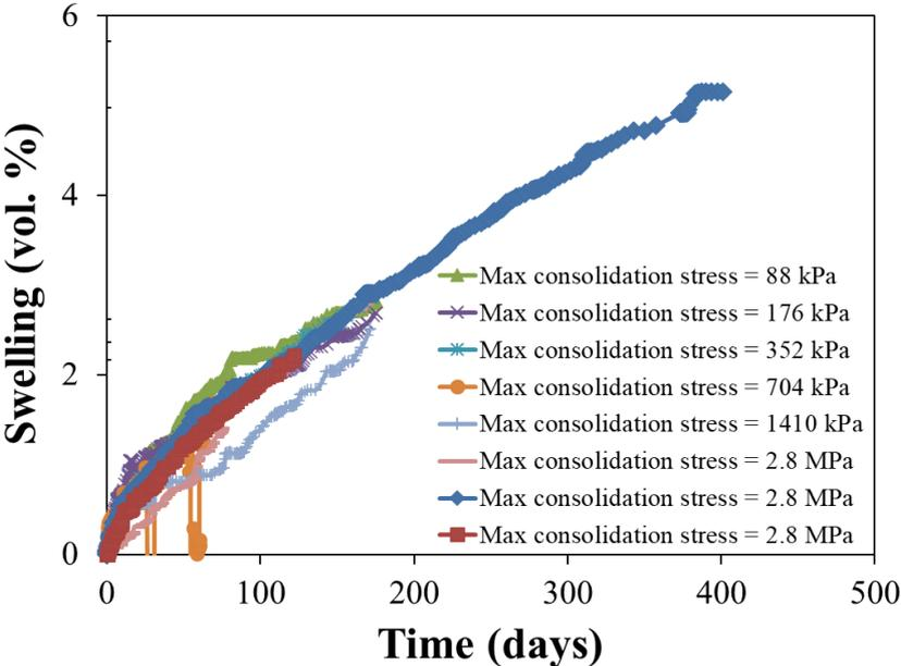
Fig. 3-17 Experimental measurements of swelling (vol. %) under 176 kPa counter-pressure on bi-salt BWPs containing 10 wt.% NaNO<sub>3</sub> and 30 wt.% of BaSO<sub>4</sub> consolidated with different level of stress.
