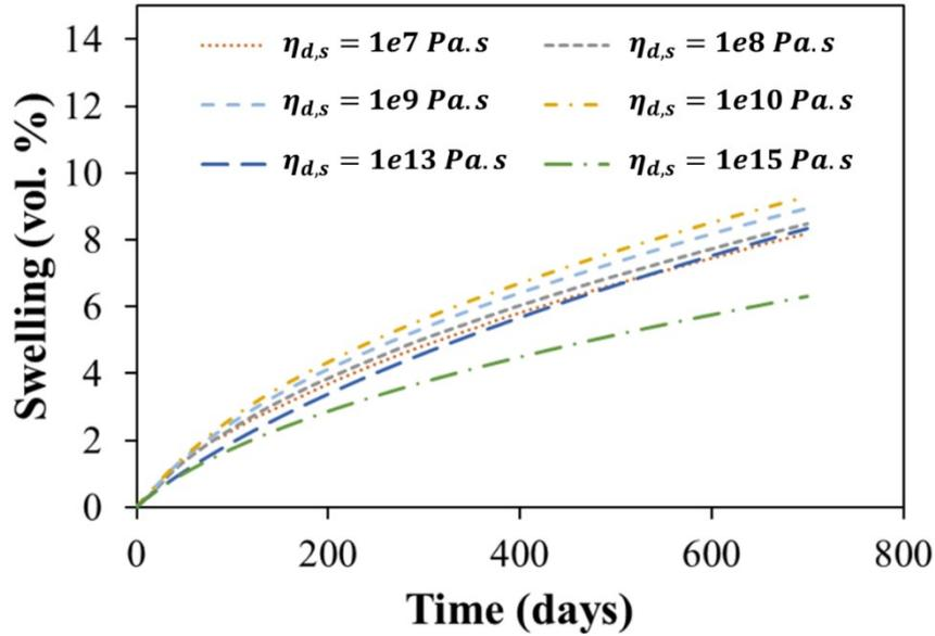
Fig. E - 4 Temporal evolutions of swelling simulated for M30\_NaNO3 BWPs under 2.8 MPa constant counter-pressure with deviatoric viscosity  $\eta_{d,s}$  ranging from  $\eta_{d,s} = 1 \times 10^7$  Pa.s to  $\eta_{d,s} = 1 \times 10^{15}$  Pa.s.
