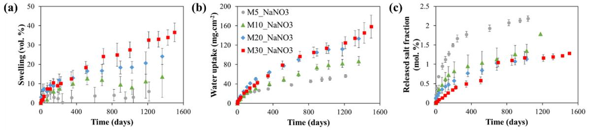
Fig. 3-4 Experimental measurements of (a) swelling (vol. %); (b) water uptake ( $\text{mg}/\text{cm}^2$ ); (c) released salt fraction (mol. %) during free leaching tests on mono-salt BWP samples containing 5 wt.%, 10 wt.%, 20 wt.% and 30 wt.% of  $\text{NaNO}_3$ .
