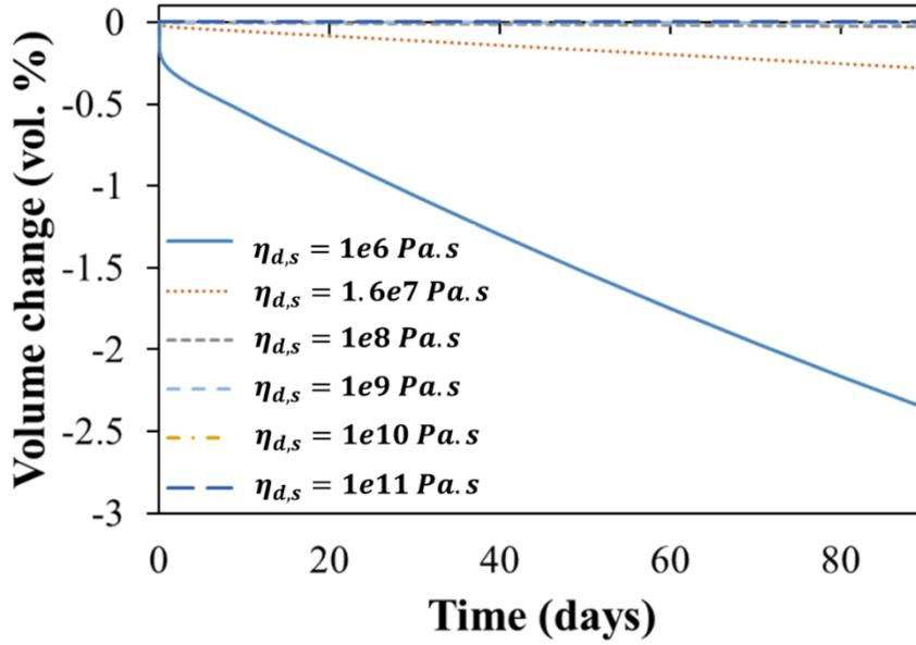
Fig. E - 1 Temporal evolutions of volume change simulated for M20\_NaNO3 BWPs consolidated under 1 Pa with deviatoric viscosity  $\eta_{d,s}$  ranging from  $\eta_{d,s} = 1 \times 10^6$  Pa.s to  $\eta_{d,s} = 1 \times 10^{11}$  Pa.s.
