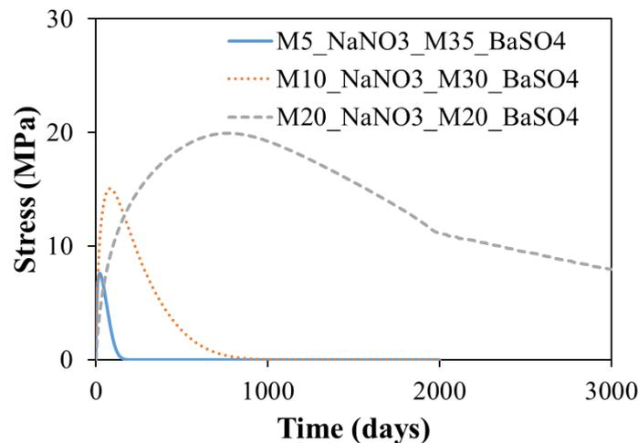
Fig. 5-35 Evolution of stress generated over leaching time within bi-salt BWPs (M5\_NaNO<sub>3</sub>\_M35\_BaSO<sub>4</sub>, M10\_NaNO<sub>3</sub>\_M30\_BaSO<sub>4</sub>, M20\_NaNO<sub>3</sub>\_M20\_BaSO<sub>4</sub>).
