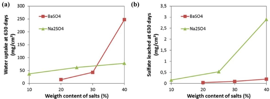
Fig. 2-8 Amount of (a) water uptake; (b) released sulfate after 630 days of leaching by pure water at 25°C for simplified BWPs containing an increasing amount of sodium sulfate  $\text{Na}_2\text{SO}_4$  and barium sulfate  $\text{BaSO}_4$  [13].
