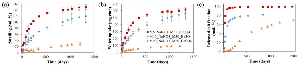
Fig. 3-7 Experimental measurements of (a) swelling (vol. %); (b) water uptake ( $\text{mg}/\text{cm}^2$ ); (c) released salt fraction (mol. %) during free leaching tests on bi-salt BWPs incorporating both  $\text{NaNO}_3$  and  $\text{BaSO}_4$ .
