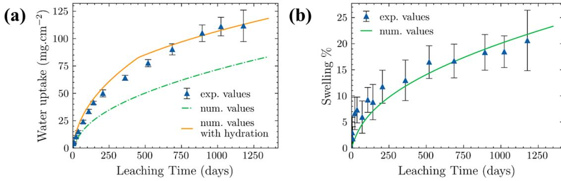
Fig. 5-5 Numerical and experimental results of the temporal evolution of (a) absorbed water; (b) swelling of M20\_NaNO<sub>3</sub> mono-salt BWP using MELOT2019 model with constant osmotic efficiency coefficient  $\tau$ .
