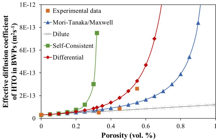
Fig. 2-12 Application of different simplified homogenization schemes in Table 9 to estimate the effective diffusion coefficient of HTO in BWPs. The experimental points are from [16] (cf. Table 7).
