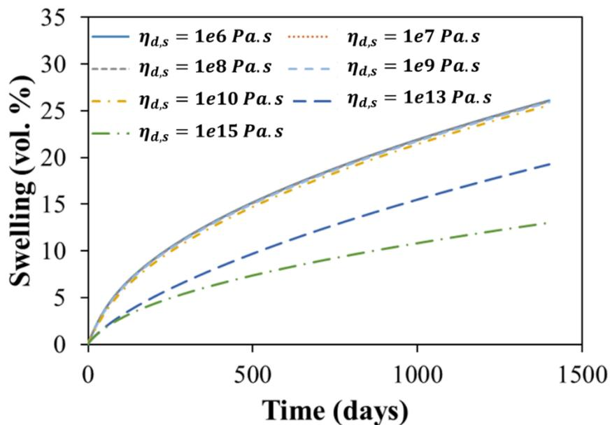
Fig. E - 5 Temporal evolutions of swelling simulated for M20\_NaNO3 BWPs under free leaching conditions with deviatoric viscosity  $\eta_{d,s}$  ranging from  $\eta_{d,s} = 1 \times 10^6$  Pa.s to  $\eta_{d,s} = 1 \times 10^{15}$  Pa.s.
