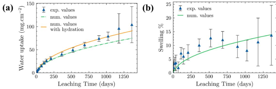
Fig. 5-9 Numerical and experimental results of the temporal evolution of (a) absorbed water; (b) swelling of M10\_NaNO<sub>3</sub> mono-salt BWP.
