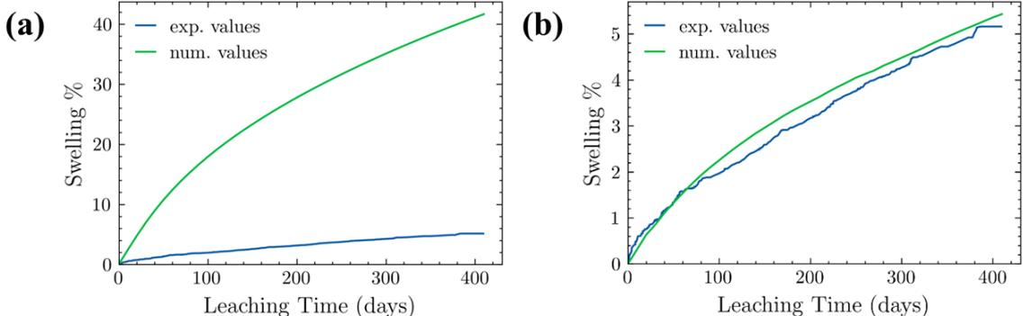
Fig. 5-27 Comparison of numerical results of  $\text{M10\_NaNO}_3\text{-M30\_BaSO}_4$  BWP swelling under 176 kPa constant counter-pressure by using parameters calibrated on (a)  $\text{M10\_NaNO}_3\text{-M30\_BaSO}_4$  BWPs (cf. Table 19) ; (b) mono-salt  $\text{NaNO}_3$  BWPs (cf. Table 18) under free leaching conditions.
