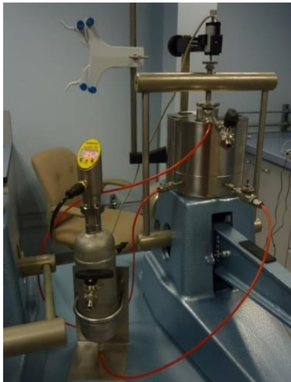
Fig. 3-3 Photo of leaching tests under constant counter-pressure - CEA.
