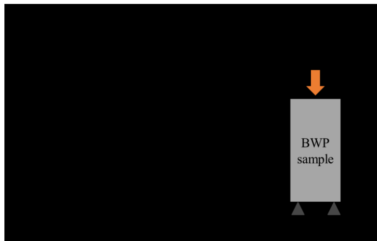
Fig. 5-21 Geometry and boundary conditions of the consolidation problem.
