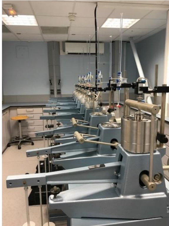
Fig. 3-2 Photo of oedometer benches - CEA.
