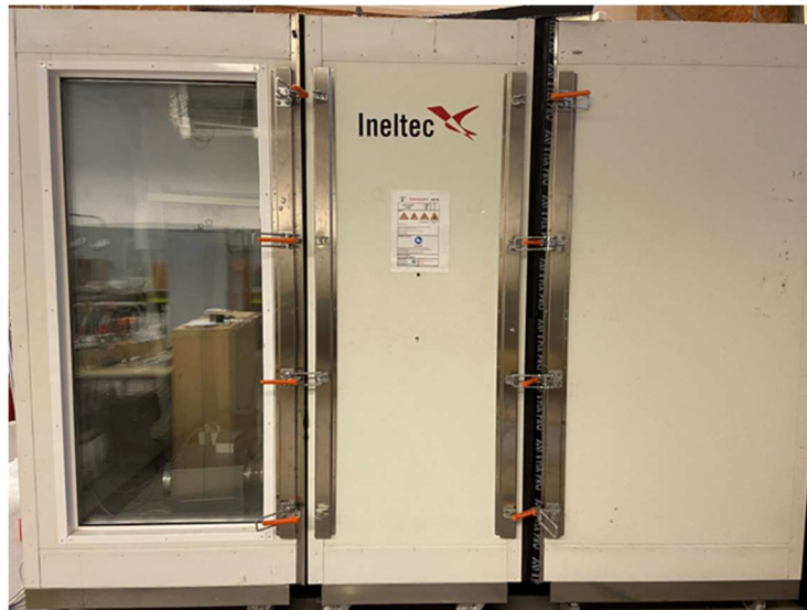
Figure 3-1 Guarded hot box in ENTPE
