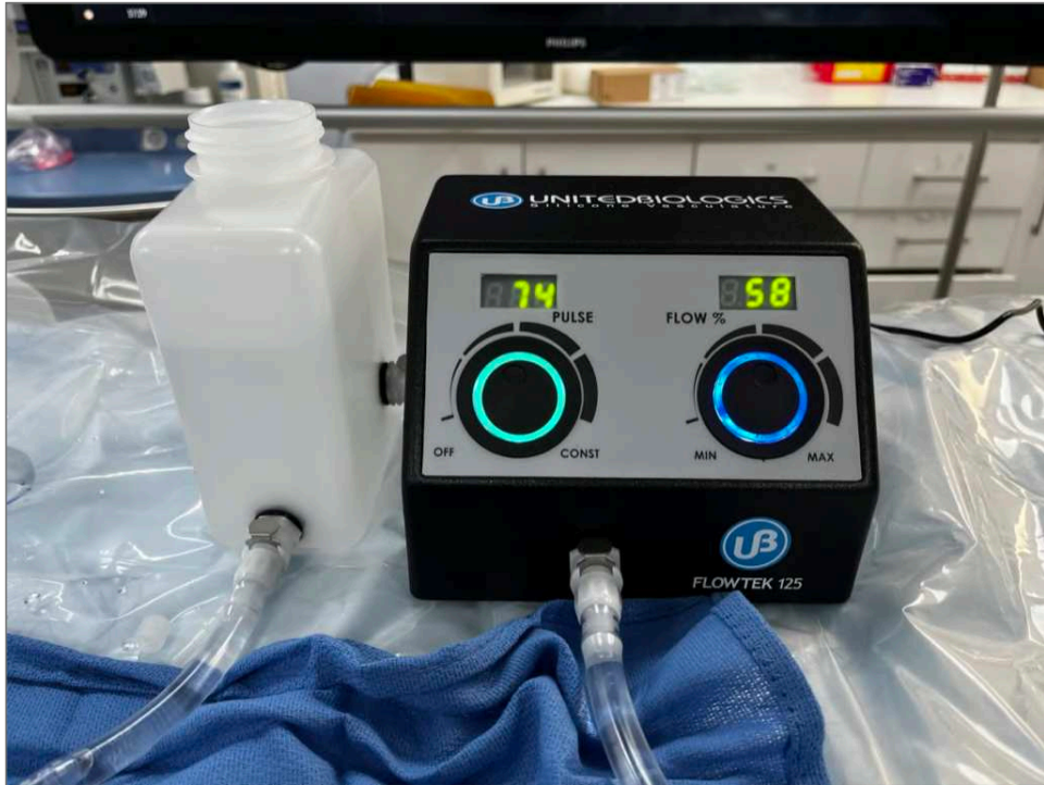
Figure 37. FlowTek 125 Pump (United Biologics Santa Ana CA USA). Image is showing the water container + pump.
