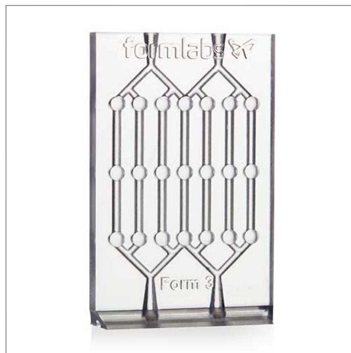
Figure 15. A millifluidic Chip printed with Formlabs 3D printer.
