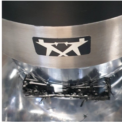
(b) Sample immersed in fluid + degassing
