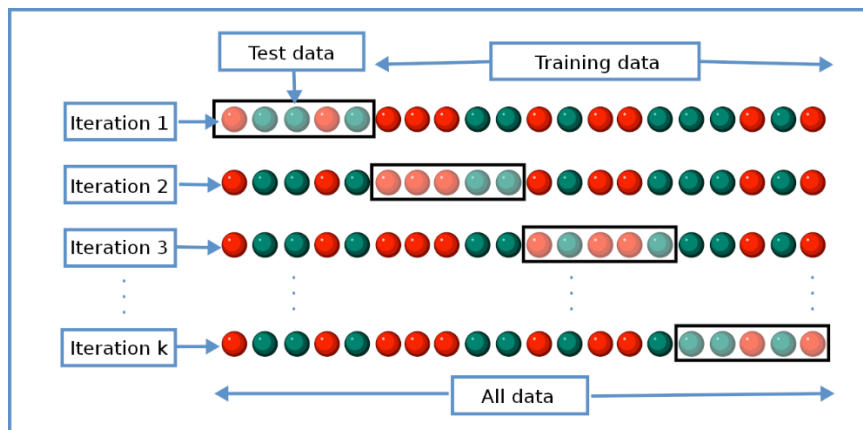
Figure 2–3: Principle of the k-fold algorithm [25].
