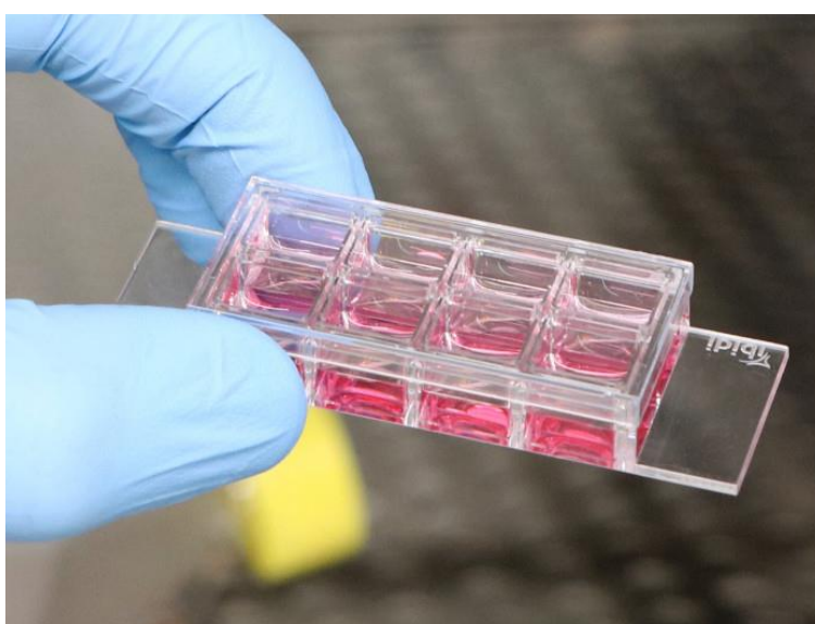
Figure 88: Ibidi® \mu -Slide 8 Well high Glass Bottom microscopy chamber. (Ibidi®)
