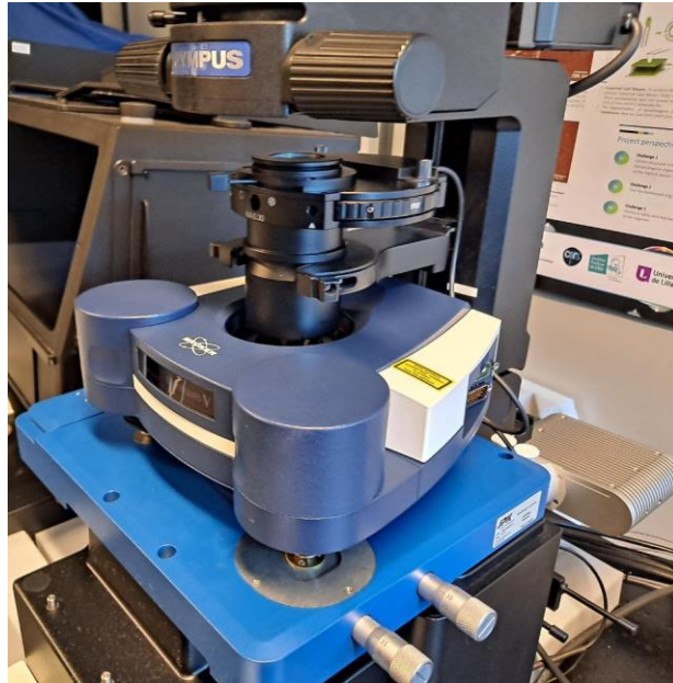
Figure 38: Example of AFM coupled to an inverted microscope. The most common technique coupled to AFM is bright-field microscopy, which allows for cantilever laser alignment, sample morphology assessment, and the selection of regions of interest to measure. Fluorescence microscopy is another widely used technique in research that complements AFM, by allowing the monitoring of biochemical processes through the labeling of specific sample components.
