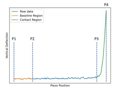
Figure 45: Diagram showing how the force curves are divided into contact and baseline regions for computing their corresponding slope.
