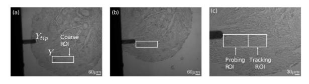
Figure 33: (a) - (c) Tracking protocol to position tissue underneath the AFM probe tip. A) The pathologist defines the ROI of interest in the sample. B) The system moves to the specified ROI and starts scanning C) within the ROI the system defines a region to measure (probing ROI) and a region to track (Tracking ROI) the position across multiple magnifications. Reproduced from (Roy et al. 2013).
