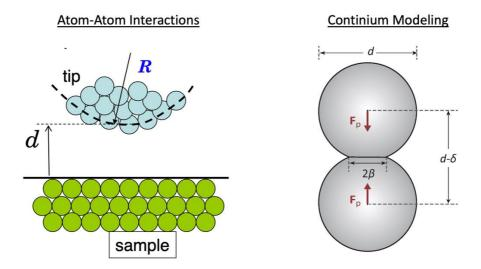
Figure 21:Diagram depicting the two main approaches to model the tip-sample interactions during an AFM measurement. Reproduced from (Raman et al. 2002 & Leduc et al. 2016)
