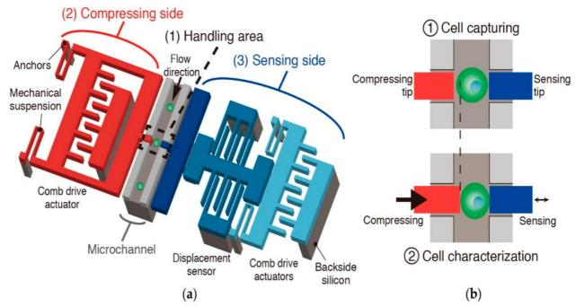
Figure 11:Diagram depicting the mechanism of the MEMS device developed by Takayama et al. 2018. This device consists of a microfluidic channel with two opposing tips to handle the cells, a series of comb drive actuators to perform compression and a differential capacitive sensor for displacement measurement. By adjusting the flow rate inside of the microchannel single cells can be captured between the sensing and compressing tip. (Takayama et al. 2018)
