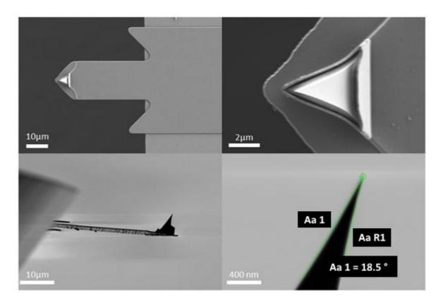
Figure 49: AC40 probe scanning electron microscopy image.
