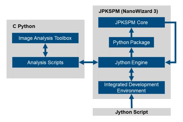
Figure 40: Diagram depicting the CPython – Jython interface developed which allows to call CPython scripts from Jython scripts while running an experiment loop in the Experiment Planner®
