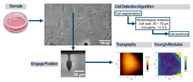
Figure 42: Diagram describing the ROI detection algorithm based on bright-field image segmentation. By applying a flat-field illumination correction and a variance filter, the ROIs corresponding to the cells are segmented from the glass. The data presented in this figure was acquired on hTERT-RPE-Icells seeded on glass-bottom petri dishes.
