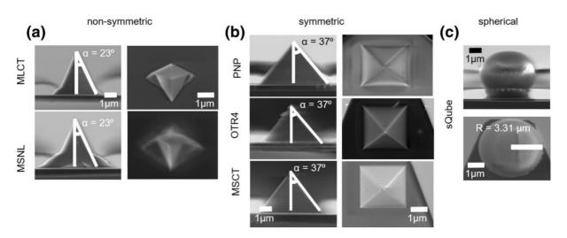
Figure 18:Examples of different AFM tip geometries. A) Non-symmetric pyramids. B) Symmetric pyramids. C) Spherical tips. Reproduced from (Zemła et al., 2020)
