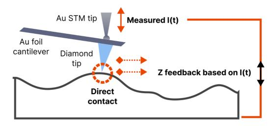
Figure 14:Experimental setup of the first AFM. An STM is used to monitor the deflection of a gold lever rastered on top of the sample surface. The tunnelling current between the gold cantilever and the STM tip (It) is used as feedback to control the sample z position.
