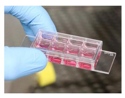
*Figure* 88: *Ibidi*® μ*-Slide* 8 *Well high Glass Bottom microscopy chamber. (Ibidi*®)
