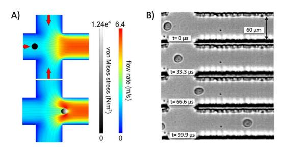
Figure 10: Microfluidic-based system developed by Belotti et al. 2019. The cells are directed into a region in the chip where a pinching flow deforms the cell. A) Diagram depicting the pinching flow and how the stress is applied on the cell. B) Optical image sequence of a cell being deformed by the pinching flow. Reproduced from (Belotti et al., 2019)
