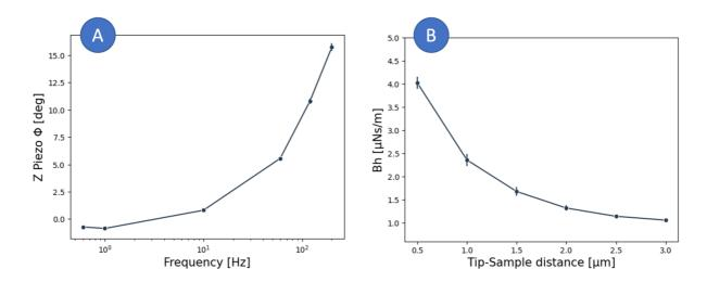
Figure 84: A) Z-piezo phase lag measured on a NanoWizard III for each frequency. B) Drag force measured at different cantilever-sample separations while applying 500 Hz oscillations. The data shown on each plot corresponds to the mean  $\pm$  SE of three 4x4 force curves maps.
