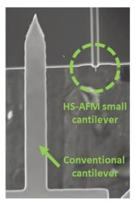
Figure 30: Examples of developments to increase AFM scan speed: Diagram depicting the optimized paths for the vertical (green trace) and horizontal (blue trace) of the cantilever in QI® mode. (Left) Size comparison between conventional cantilevers and small cantilevers used in HS-AFM (Right).
