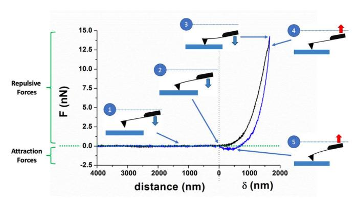
Figure 20:Summary of tip-sample force vs tip-sample distance curve acquisition by AFM. 1) The cantilever approaches the sample surface. 2) The AFM-tip contacts the sample surface. 3) The force (F) / indentation ( $\delta$ ) setpoint is reached. 4) The cantilever starts to retract from the sample surface. 5) The maximum attraction force is sensed by the cantilever before detaching the sample. Image modified from (Gavara, 2017).
