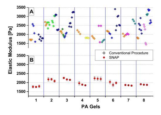
Figure 29: Comparison of the Elastic modulus measured on polyacrylamide (PA) gels by different labs and by different users on different instruments. The SNAP calibration method greatly reduces the variability between measurements when compared to the conventional calibration procedure. (Schillers et al. 2017)
