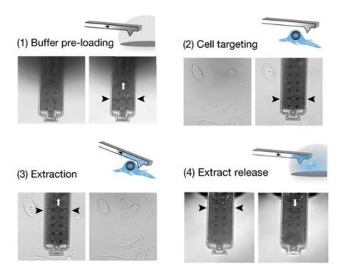
Figure 27: Diagram summarizing the principle of Live-seq using FluidFM. 1) The microchannel inside of the cantilever is loaded with buffer. 2) The user selects the cell from the sample. 3) The sample is extracted from the cell. 4) The extract from the cell is released. Reproduced from (W. Chen et al., 2022)
