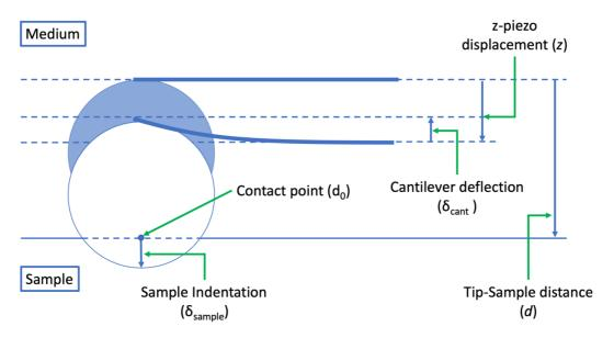
Figure 19:Diagram depicting an AFM tip indenting the sample with the nomenclature normally used to describe the physical variables involved in the process.
