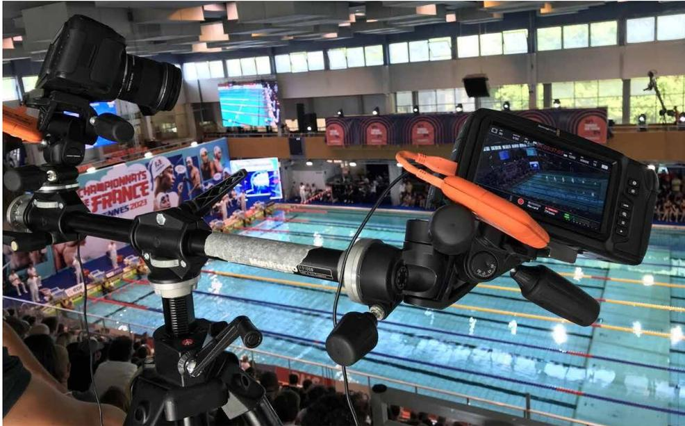
Figure 5.5: Video recording setup: left and right cameras independently recorded half of the pool.
