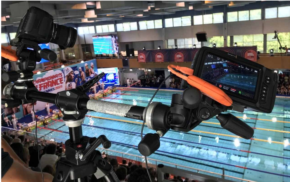
Figure 5.5: Video recording setup: left and right cameras independently recorded half of the pool.
