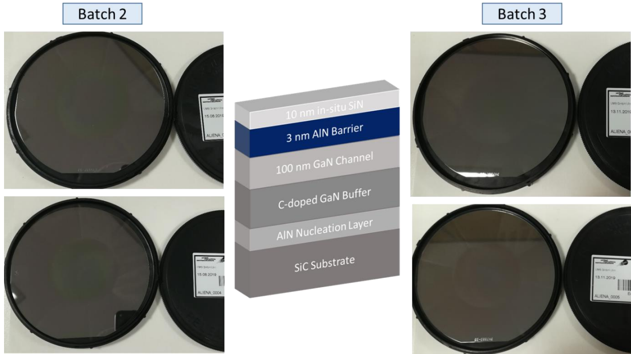
Figure.3.36. Schematic cross section and photos of the 3 nm AlN/GaN heterostructures
