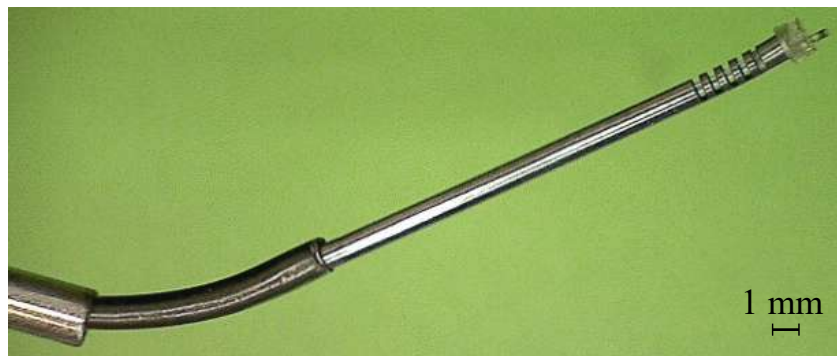
FIGURE IV.19 – Hybrid CTR is built according to the simulation results. The laser optical fiber protrudes about 1 mm from the outside of the end cap. The outer and inner diameters of the three tubes are: 2.50 and 1.80 mm, 1.50 and 1.25 mm, 1.08 and 1.00 mm,
