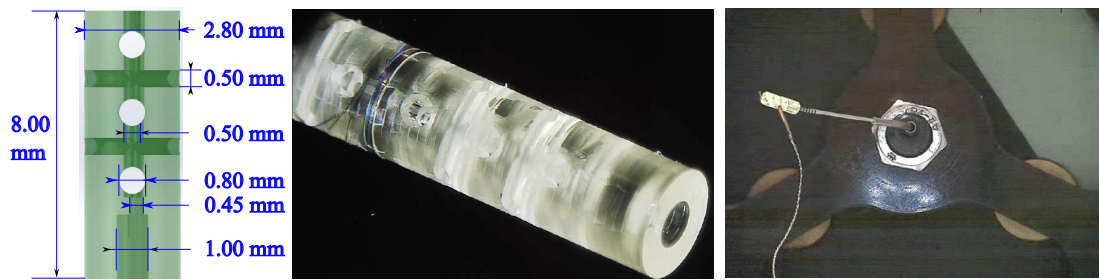
FIGURE V.8 – Nanoscribe 3D printed end cap of the wrist dedicated to the integration of the AURORA magnetic sensor.
