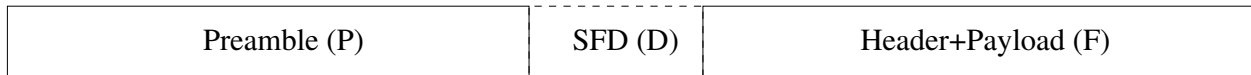
Figure 4.10: The structure of a LoRa frame according to the type of chirps: up-chirps are used for the beginning of the preamble, down-chirps for the end of the preamble, and up-chirps for the header and payload.
