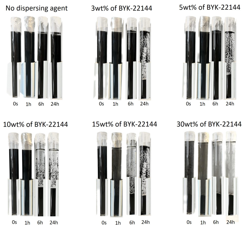
Figure 5.7: The sedimentation experiments conducted on CB powder with varying quantities of BYK-22144.
