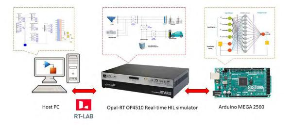
Figure.39 The Hardwar-In-th-Loop configuration.
