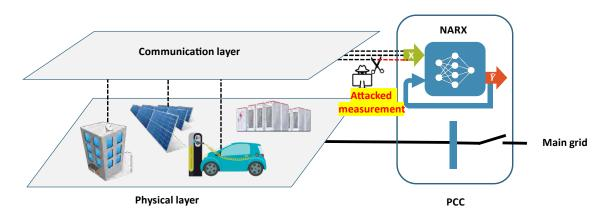
Figure.27 Cyber-attack on the transmitted measurements.
