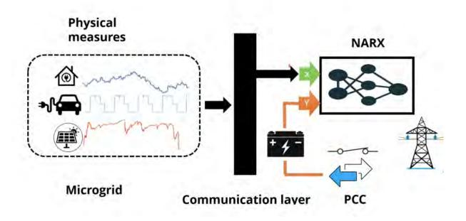
Figure.21 The NARX Input and target in the training phase.
