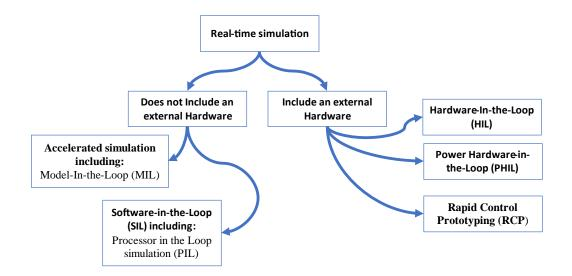
Figure.8 Real-Time simulation branches.
