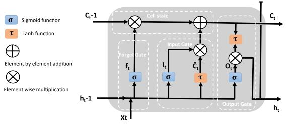
Figure.49 LSTM Cell.
