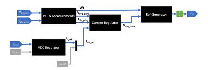
Figure.16 Control algorithm of the PV inverter.
