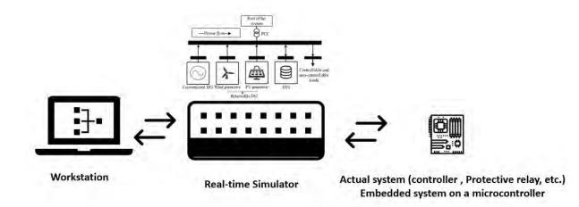
Figure.10 Hardware-In-the-Loop (HIL) configuration.
