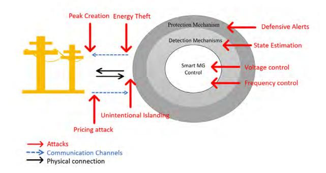
Figure.5 Cyber-attacks on smart microgrids.
