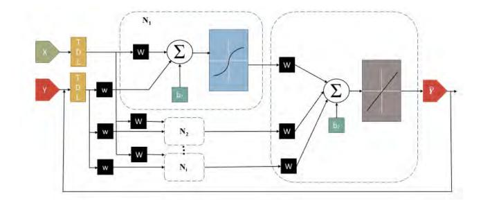
Figure.18 Detailed cross-section structure of the used NARX.
