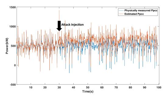
Figure.29 FDI attack: injection of higher production PV profile.
