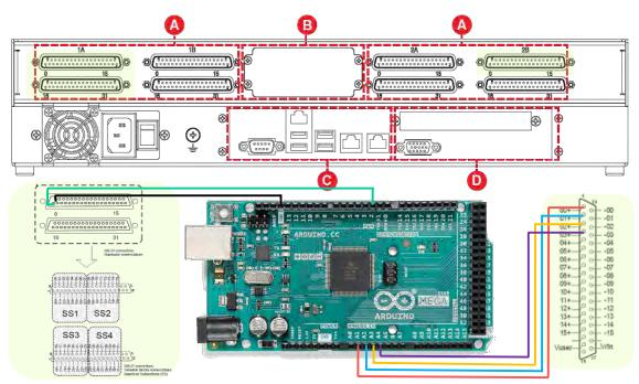
Figure.42 Connections between the Arduino board and IO opal interface.
