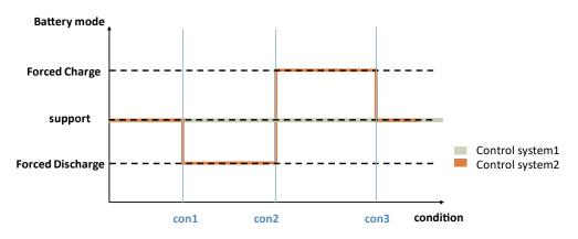
Figure.45 Different Battery control systems.
