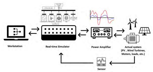
Figure.11 Power Hardware-in-the-Loop (PHIL) configuration.
