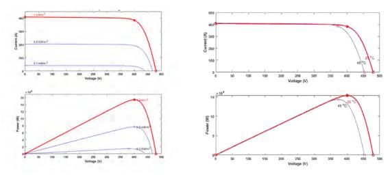
**Figure.15** PV sub-array (I\_V) and (P\_V) for solar irradiances (0.1 kW/m<sup>2</sup>, 0.5 kW/m<sup>2</sup>, 1 kW/m<sup>2</sup>) and temperatures (25°C, 45°C).
