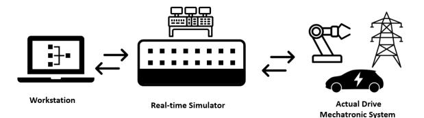
Figure.12 Rapid Control Prototyping (RCP) configuration.
