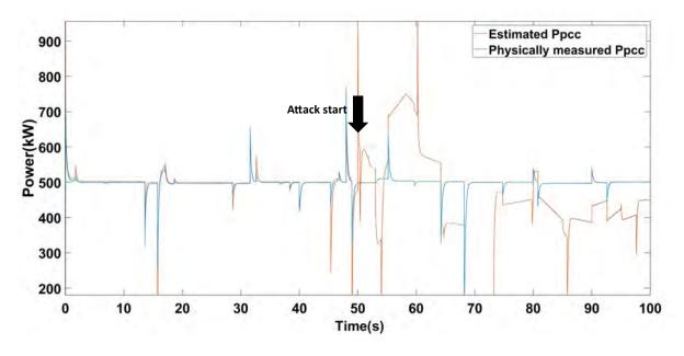
Figure.33 Dos attack: Delayed BMS reference signal.
