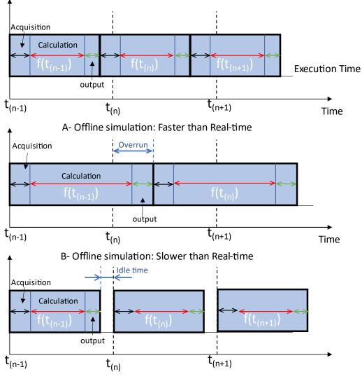
C- Real-Time simulation: Synchronized
