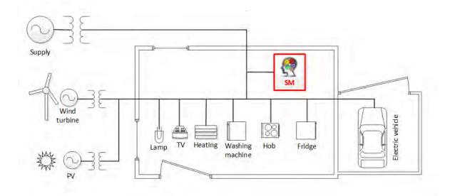
Figure.3 Smart meter connection.
