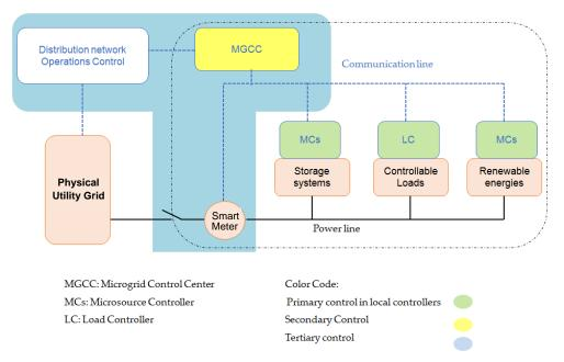
Figure.4 Modern basic structure of a microgrid.
