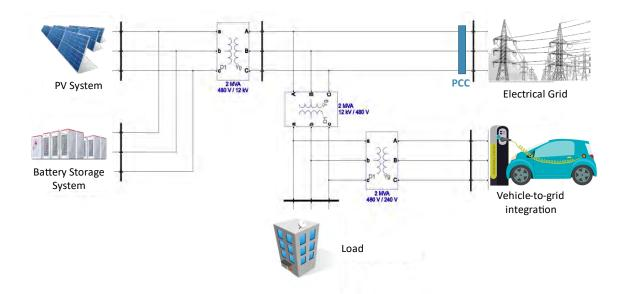
Figure.14 The used microgrid components: Case (A).
