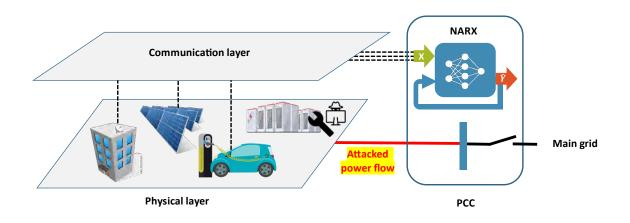
Figure.28 Physical attack on the BMS.
