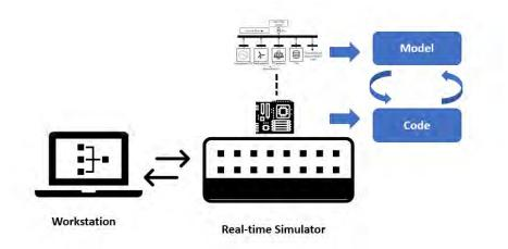
Figure.9 Simulation-In-the-Loop (SIL) configuration.
