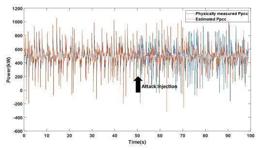
Figure.31 FDI attack: injection of replayed (repeated) PV profile.
