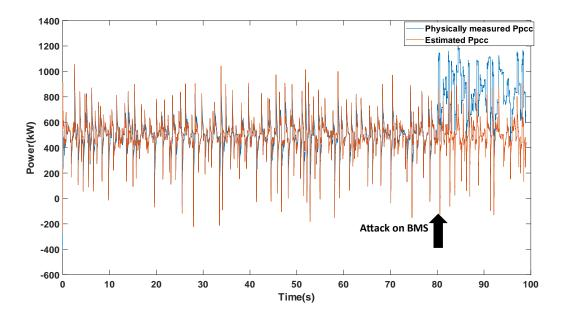
Figure.37 Forced discharging attack on the battery at ts=80 s.
