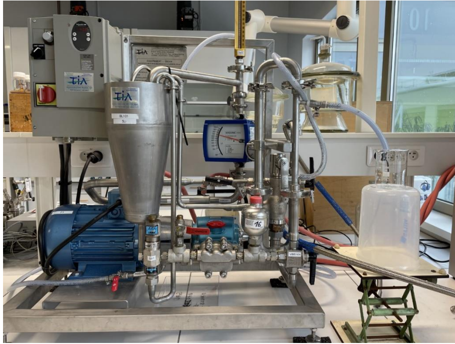
Figure II-1: Setup of the ultrafiltration pilot-plant.
