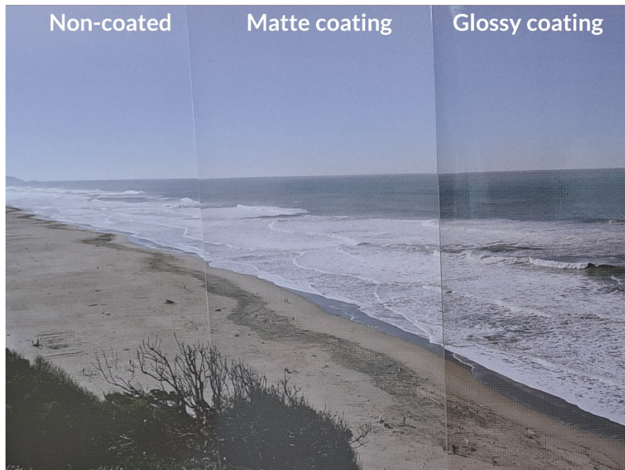
Figure 1. Picture printed in inkjet on a glossy photo paper. The left part is non-coated, the middle part is coated with a matte-finishing layer, and the right part is coated with a glossy-finishing layer.
