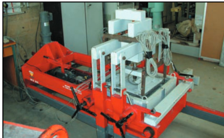
FIGURE 5.4: The direct shear test (Reiffsteck et al., 2007)
