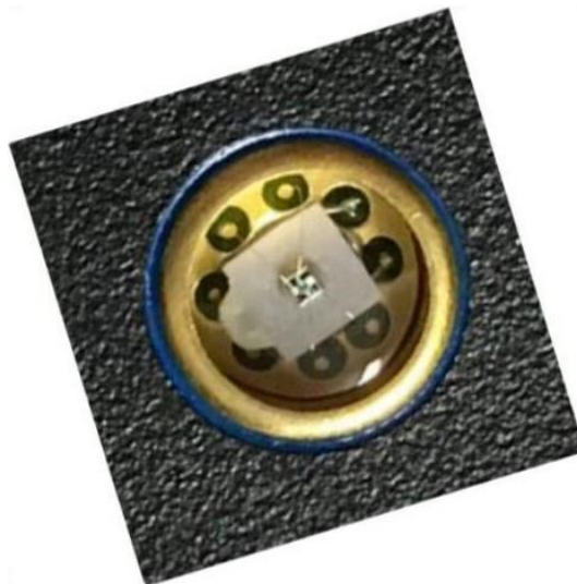
Figure 7.34 Picture of the SPAD front side, showing the sensitive area and the surrounding window.
