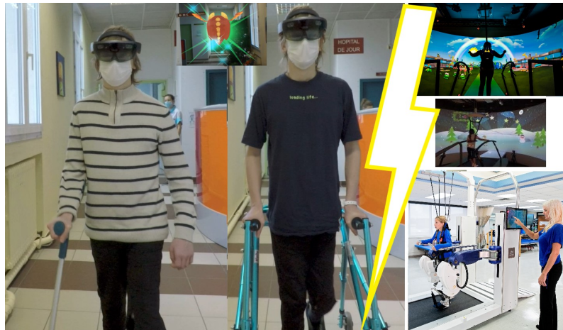
Figure 2.12 – Overground Gait Training in AR vs. Treadmill Gait Training in VR. On the left, overground gait training with an AR headset (extract of the ARRoW-CP AVG), child is free to walk in the real environment using her/his walking aids. On the right, treadmill gait training with the Motek GRAIL system with body-weight support and walking constraints due to the treadmill
