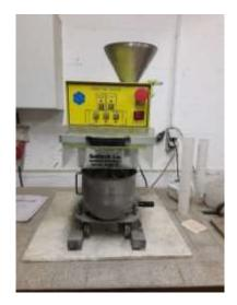
Figure 40: Standard cement paste preparation mixer
