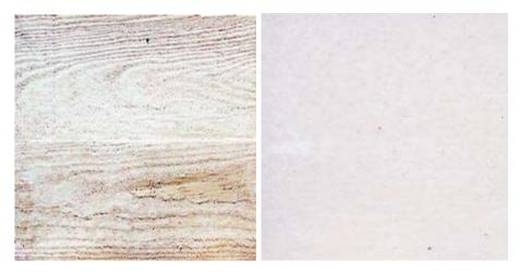
Figure 31 Two surfaces made with an identical concrete composition and casting procedure, but different formwork [126]
