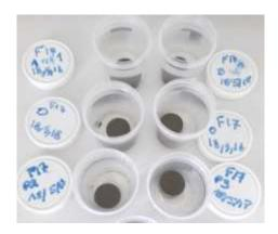
Figure 48 Cement paste sample in the acetone
