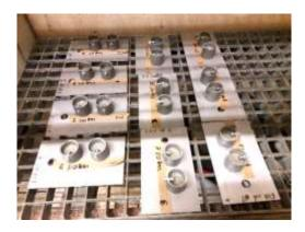
Figure 44: Curing of the cement paste samples in the chamber
