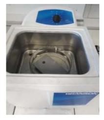
Figure 50: Ultrasonic bath apparatus containing a solution of 50% distilled water + 50% ethanol.
