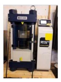
Figure 46: Compressive test machine
