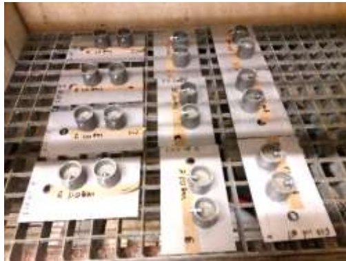
Figure 44: Curing of the cement paste samples in the chamber
