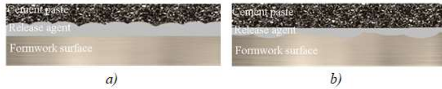
Figure 93 Effect of release agent using on : a) smooth formwork on the micro-roughness of the surface of the cement paste, b) rough formwork on the microroughness of the surface of the paste
