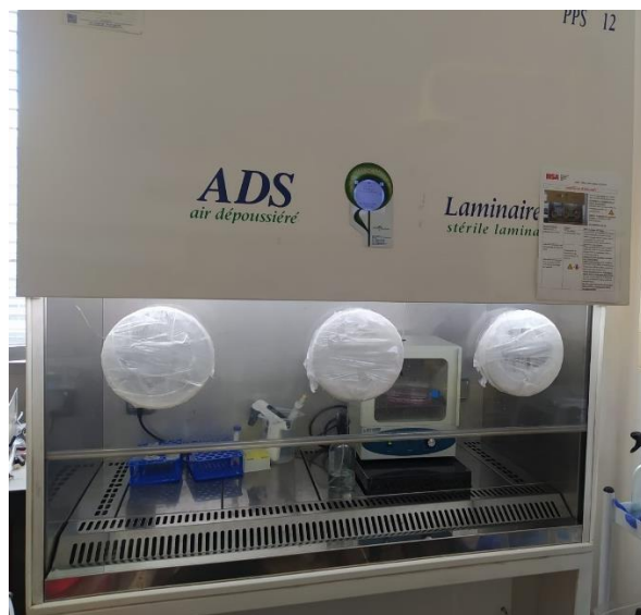
Figure 132 Class II hood used to perform all the cells manipulation.
