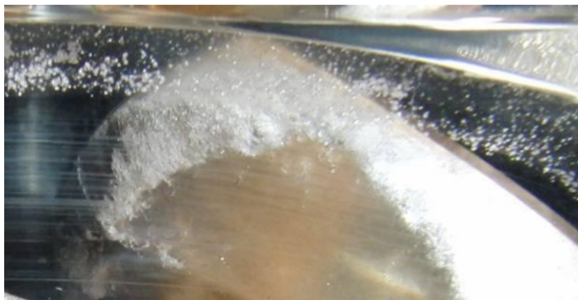
Figure 1.16 Leading edge cavitation [14].
