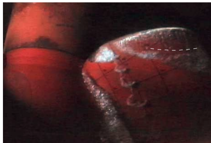
Figure 3.2 Experimental observation of the hub and the leading edge cavitation by Grekula and Bark [74].
