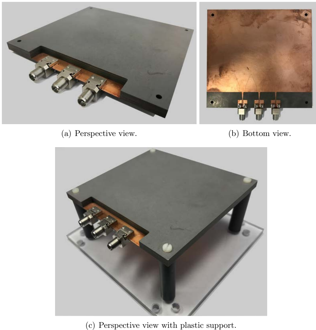
FIGURE 6.19: Photographs of the fabricated prototype. (a) Perspective and (b) bottom views. (c) Antenna adjusted on a plastic support.
